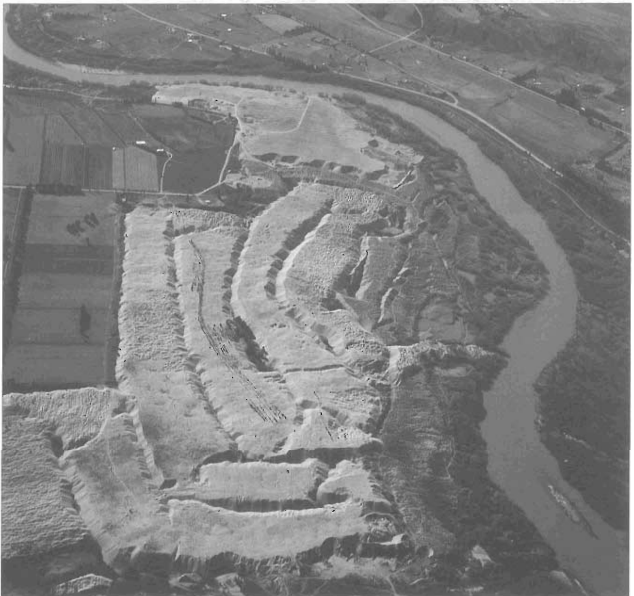
Earsclengh Flat Dredge tailings. The broad pale bands are the tracks of the Clutha Dredge formed in the middle of the 20th century. The dredge entered from the river just right of centre of the photograph. The darker ground between the pale bands and the river are the tailings left by two or three smaller dredges at the beginning of the century. Photograph: Kevin Jones, DOC
