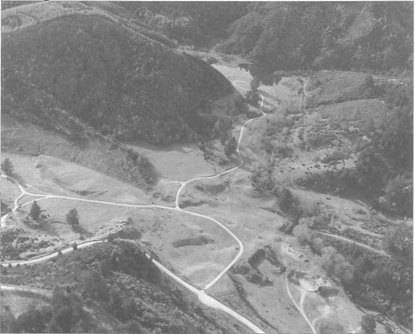
reservoirs for the pipes to the hydraulic elevators that dug out the valley in the right middle ground. An entrance to a kilometre of tunnels in the cemented conglomerate lies under the trees at the far left.
