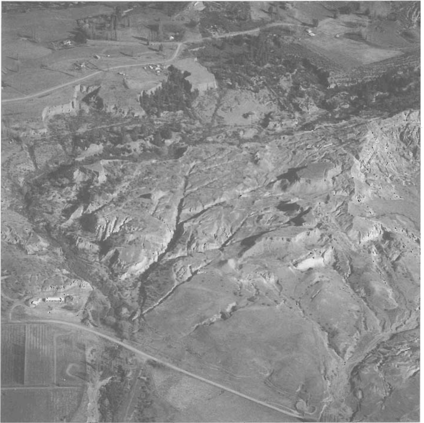
Two photographs of the Bannockburn sluicings. Two major reservoirs (Tippett's and Carrick) are high centre, with lines of distributor races marked by briar rose bushes running along the terrace to the cliff edge on the left. Rivetted pipes would have led
