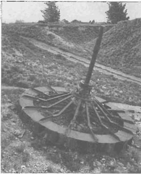
A silt wheel from the Earnsclough No. 3 dredge which was used to get rid of fine material.
