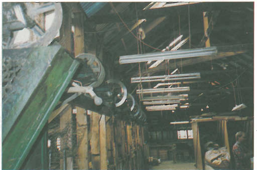
The Shag Valley station woolshed still has Lister shearing machines, which were installed in the 1920s. There is a flywheel above each shearer (and a modern fluorescent light).
