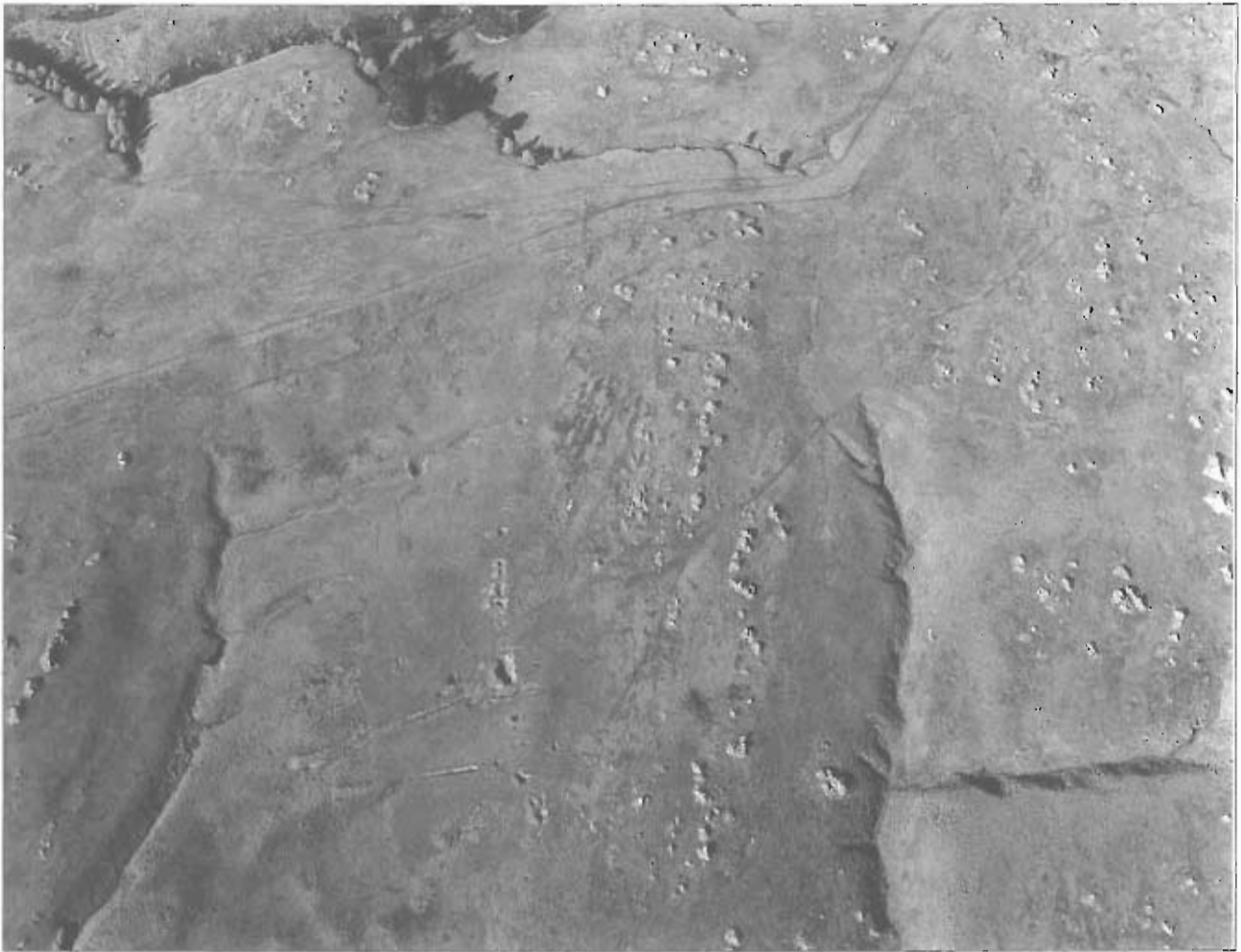
Barewood quartz mine, showing trenches and shafts aligned along the reefs.
