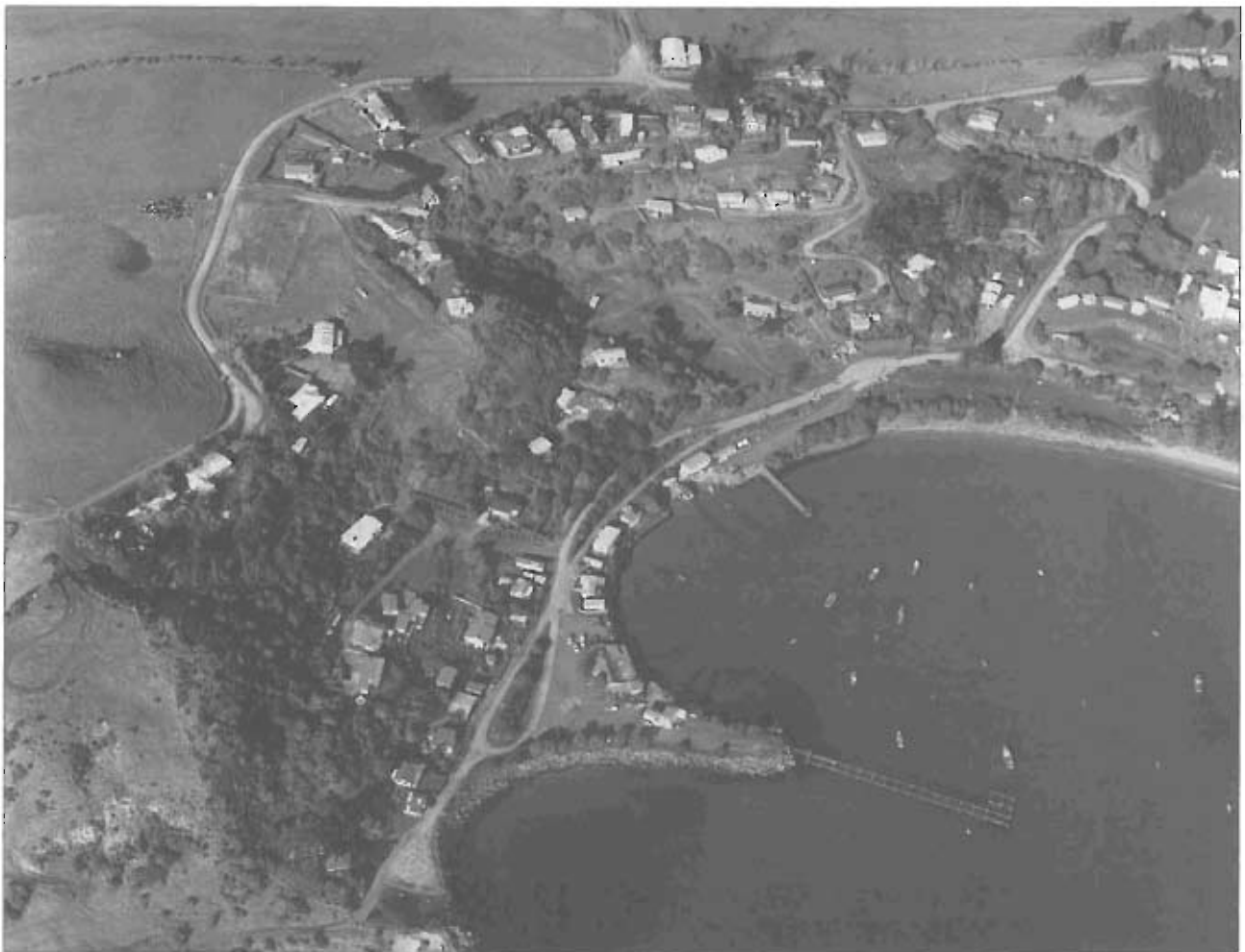
Moeraki. The whaling station lay in the curve of the bay. The iron wharf was built in 1873, but the port never achieved its potential, mostly because unstable ground along the shoreline prevented the development of onshore facilities.
