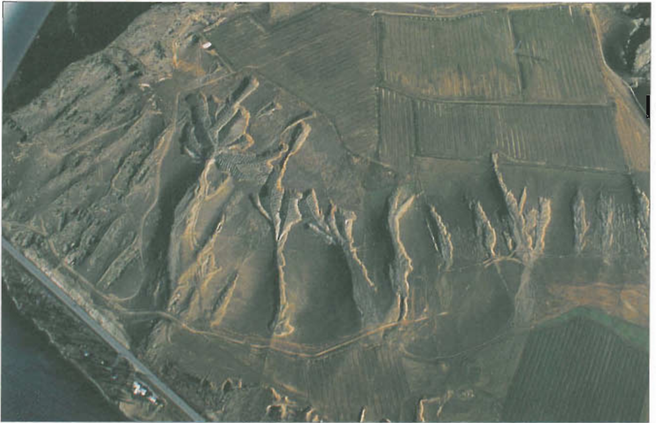
Northburn herringbone tailings which were drained down to the Clutha River in the foreground. Scraping with a grader to form border dykes has destroyed the head races and reservoirs in the background.
