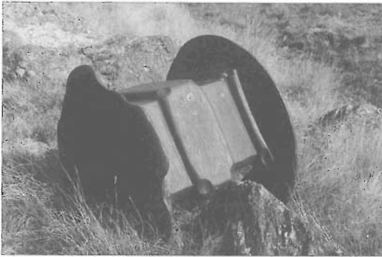
An angular dredge tumbler, over which the buckets jerked to shed their load. This one was lying on the flats of the Lower Nevis and was probably discarded by the Lower Nevis Dredge.
