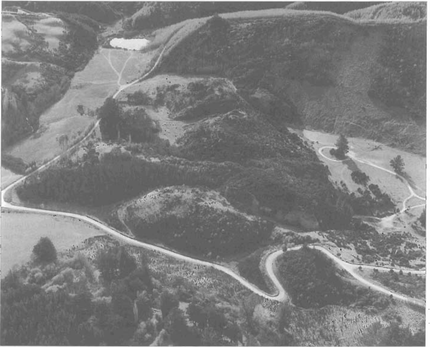
Gabriels Gully. The Blue Spur runs from the left foreground to the steep bare slope in the middle background. This slope is a slickenside fault formation uncovered by sluicing. Under the trees at its left-hand end, five large parallel races were dug to act as
