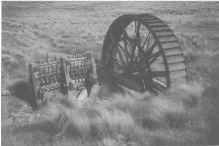
The Serpentine Battery in its final resting place. It is the only battery in Otago with its driving water-wheel still beside it.
