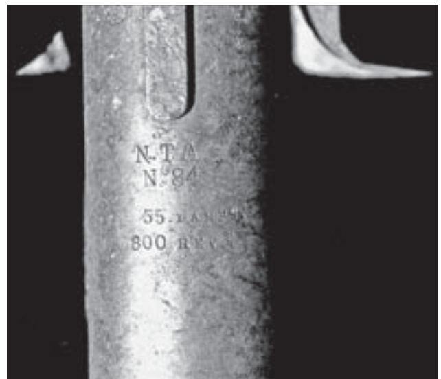
Figure 29. Dynamo shaft, showing speed and output markings.
