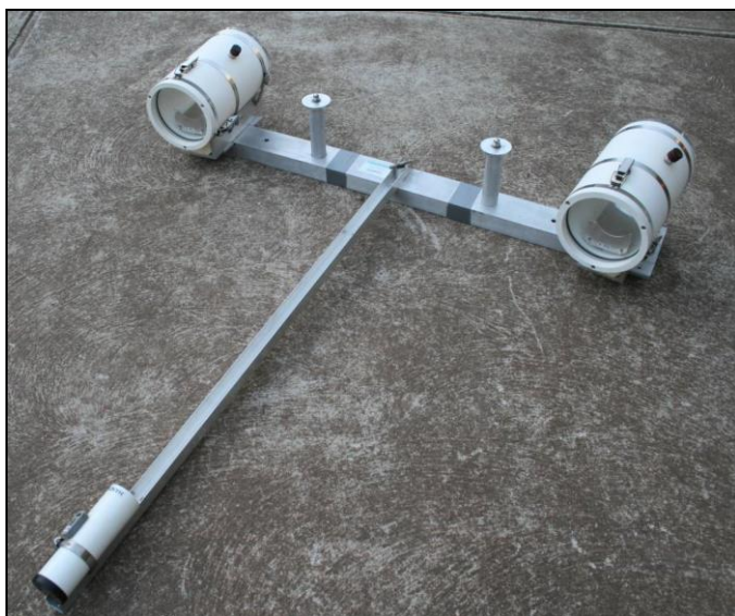
Figure 3. A stereo-video system. Note the diode (white) at the front of the system, which allows the left and right camera to be synchronised. Newer systems do not need the synchronising diode anymore. The two housings hold the video cameras. Photo credit: SeaGIS.
