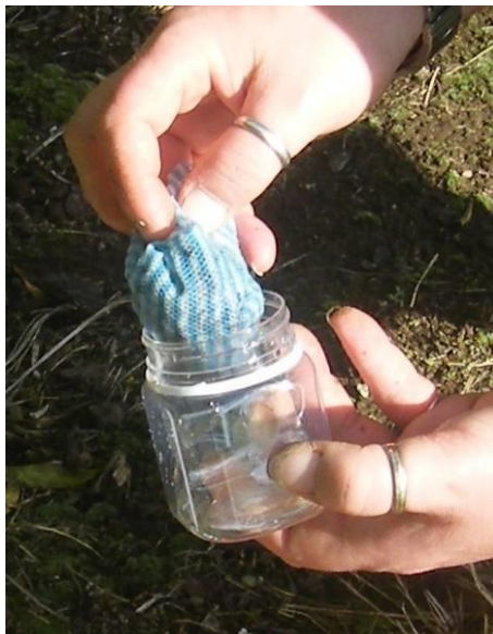
Figure 9. Pick up the Chux multifold cloth by the four corners and drop it and the strained material into a collection container (left). Write out the label (right) and place it in the container so it can be read from the outside.
