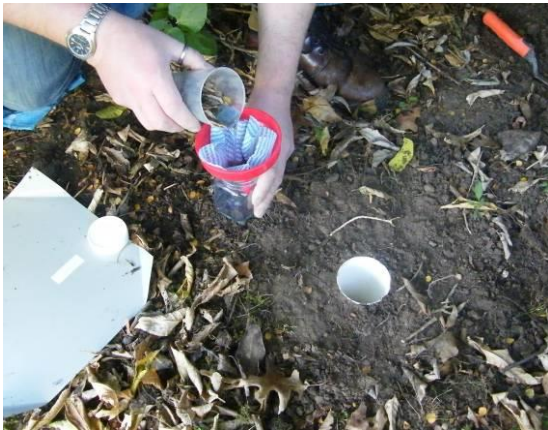
Figure 8. Sample collection. Remove the cup and strain the contents through the Chux multifold cloth (left) then repeatedly return the strained fluid back into the jar, swish it around and strain it again (right) until the sample jar is clean. Remove any large sticks or leaves from the material in the Chux multifold cloth, making sure no invertebrates are attached to them.
