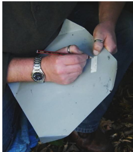
Figure 9. Pick up the Chux multifold cloth by the four corners and drop it and the strained material into a collection container (left). Write out the label (right) and place it in the container so it can be read from the outside.
