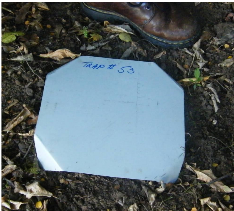
Figure 7. Write the trap number on the cover and if using an aluminium cover, complete the trap by placing a small weight on it (not shown).
