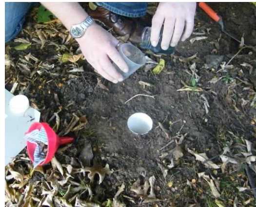
Figure 8. Sample collection. Remove the cup and strain the contents through the Chux multifold cloth (left) then repeatedly return the strained fluid back into the jar, swish it around and strain it again (right) until the sample jar is clean. Remove any large sticks or leaves from the material in the Chux multifold cloth, making sure no invertebrates are attached to them.
