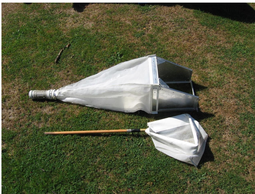
Figure 3. The kick-net (bottom) compared to a Surber sampler. Note triangular net with reinforced outer rim to prevent undue wear during sampling.
