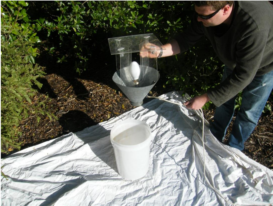
Figure 2. A modification of a light trap for catching live insects when an attendant is absent. Note that the bucket should be filled with loosely packed crumpled newspaper and that this trap is not very efficient in windy conditions unless the bucket is set into the ground.
