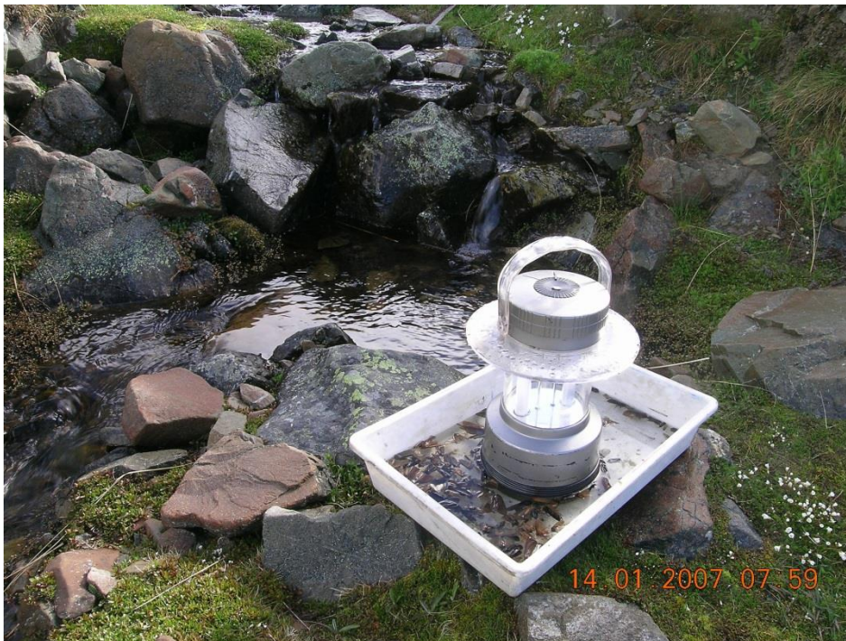
Figure 3. Portable battery-operated light trap. This light trap uses a commercially available lantern with one of the fluorescent light tubes replaced with a UV one. Note that this light trap is used with a pan of soapy water for collecting the insects. The soap causes the insects to sink after which they soon stop struggling. However, the insects will remain alive for many hours and even moths will fly off again after they dry out.
