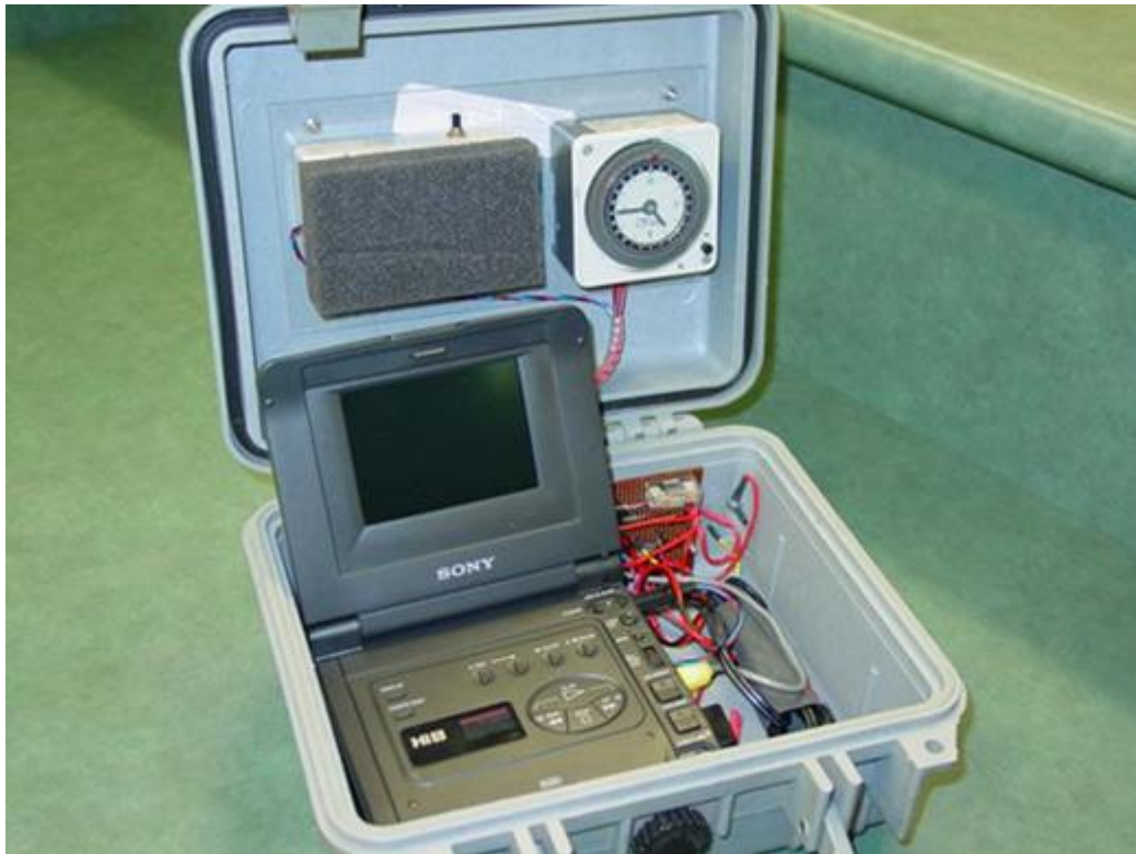
Figure 8. Sony Video-Walkman housed inside a 'Pelican' brand case with standardised waterproof 'Amphenol' brand plug and socket connectors for the camera and lights. An additional timer system has also been wired inside the case.
