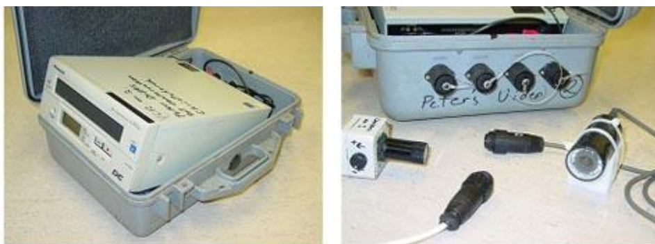
Figure 7. Panasonic 12 V video recorder (AG-1070DC), housed inside a 'Pelican' brand case with standardised waterproof 'Amphenol' brand plug and socket connectors for the camera and lights.
