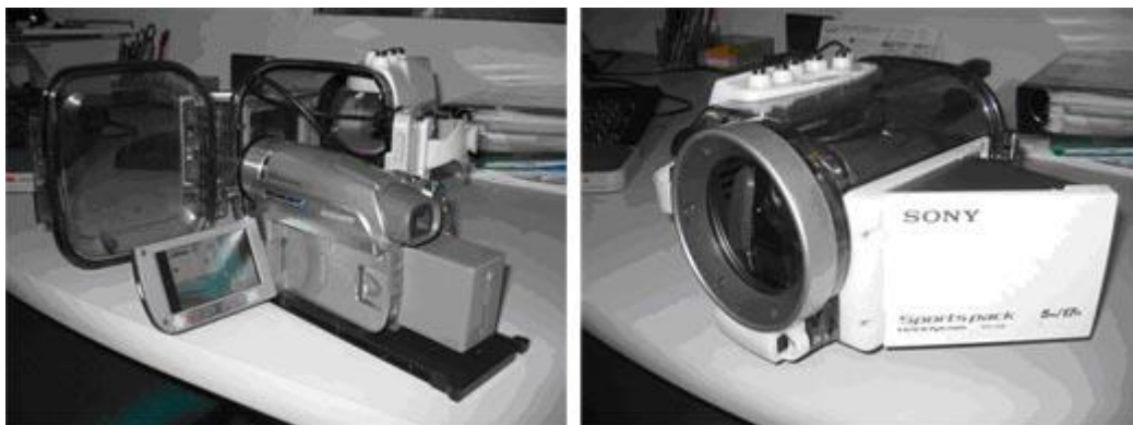
Figure 9. Small hand-held video camera with waterproof housing.
