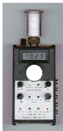
Figure 7. Examples of detectors that use different methods for transforming ultrasound into audible sound.
