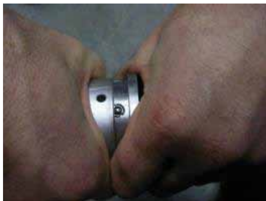
Figure A1.1. Removing the cover of the recorder.
