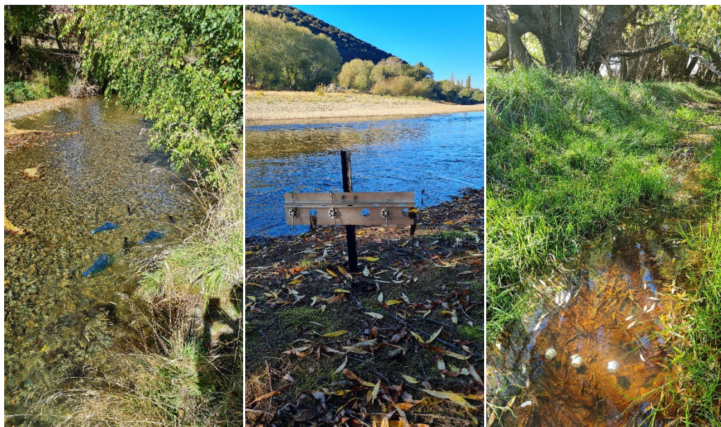
Figure 3: The three passive eDNA samplers used in this study include the bag design (left), pods mounted to a mount (middle) and pods mounted directly into the sediment (right).
