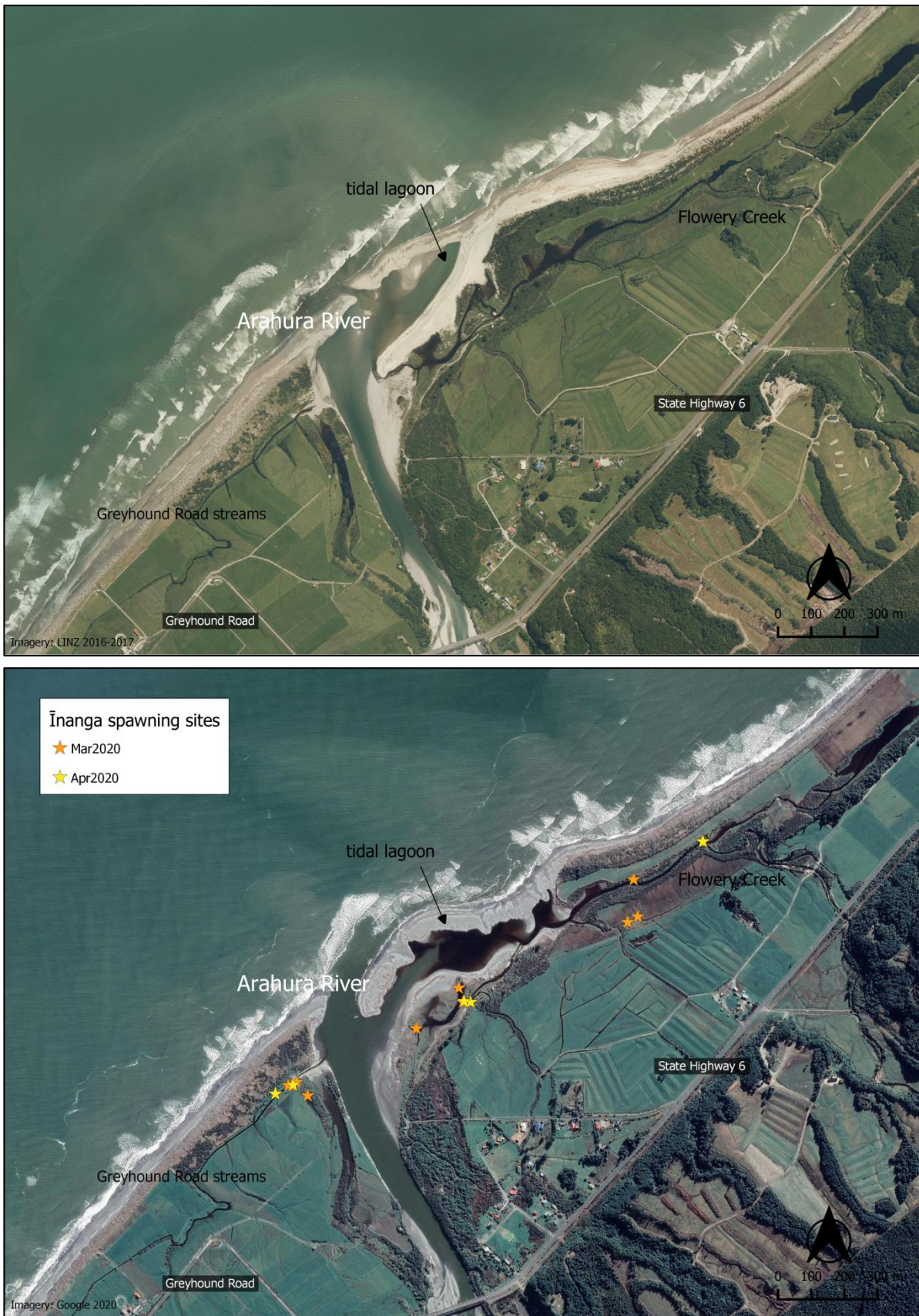
Fig. 10. Changes to the tidal lagoon system between the summers of 2017 (top) and 2020 (bottom), as seen in satellite imagery. The location of Īnanga spawning sites recorded in 2020 is shown for comparison in the lower image. Note changes in connectivity to the Flowery Creek tributaries associated with major erosion and enlargement of the tidal lagoon on its eastern shoreline.
