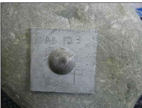
Figure 32. Corner markers. 10 mm flat head washer bolted to a rock with 8 mm galvanised coach and with plot identifier engraved.
