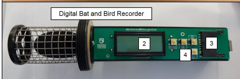
Figure 36.d Non-directional the dual acoustic and bat recorder (electronics view).
