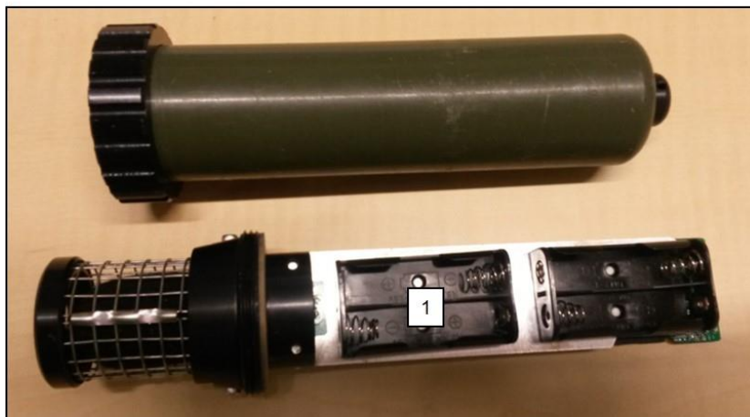
Figure 36.b Non-directional bat recorder (battery view).
