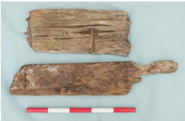
Figure 84. Piece of timber with a treenail (a type of wooden fastening used in boat building), 2018. Photo: Peter Petchey.
