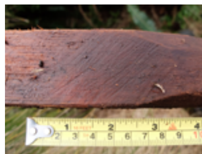
Figure 153. Hand saw marks on one face of the South Bay fingerpost, 2018. Photo: Peter Petchey.
