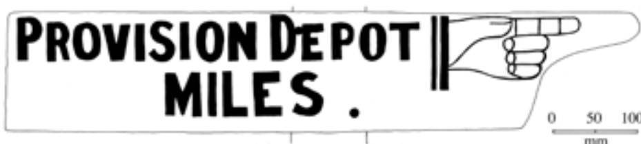
Figure 129. Tracing of the raised Alert Bay fingerpost 2018. Note that the actual number of miles to the depot would have been added in a different paint when the post was erected, and eroded away more quickly than the other signwriting, thus providing less protection to the wood beneath.
