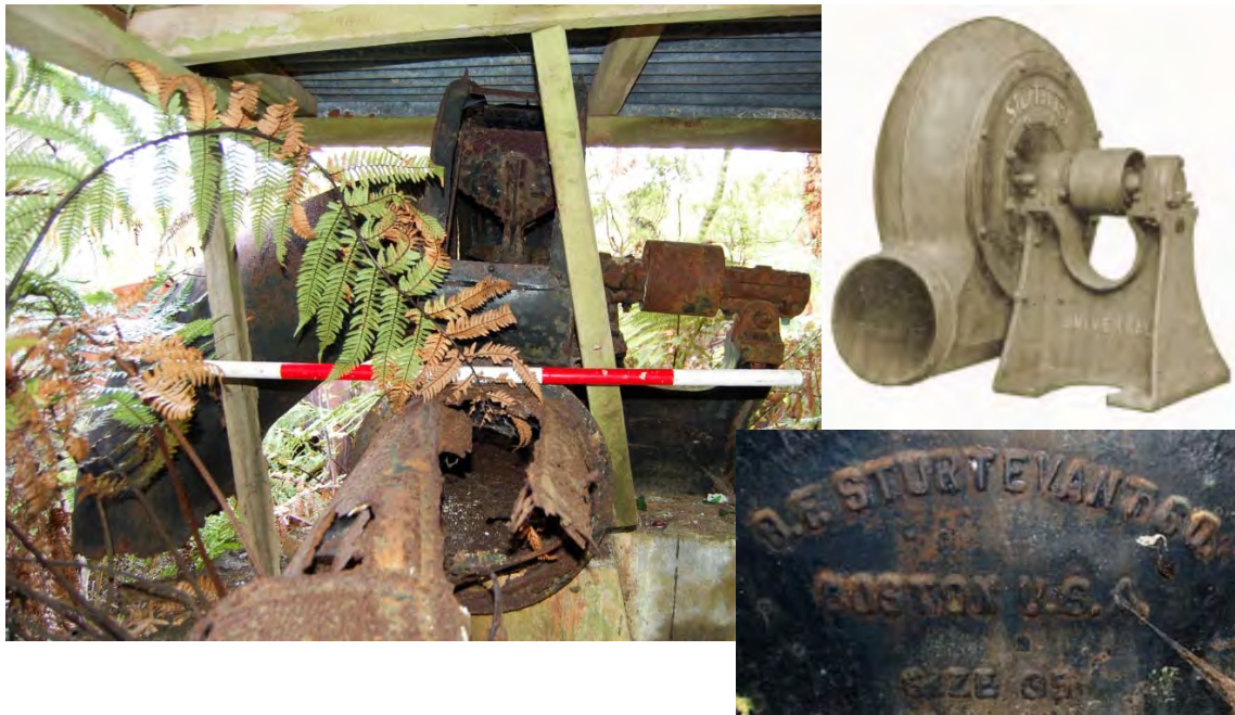
Figure 5: cast iron Sturtevant fan under rough corrugated iron roof. “Monogram” model, manufactured in the 1920s – 1940s. A large volume fan, adapted for exhausting smoke fumes and gasses from engine-rooms, laboratories and kitchens (see B. F. Sturtevant, n.d., and also www.sturtevantfan.com ).
