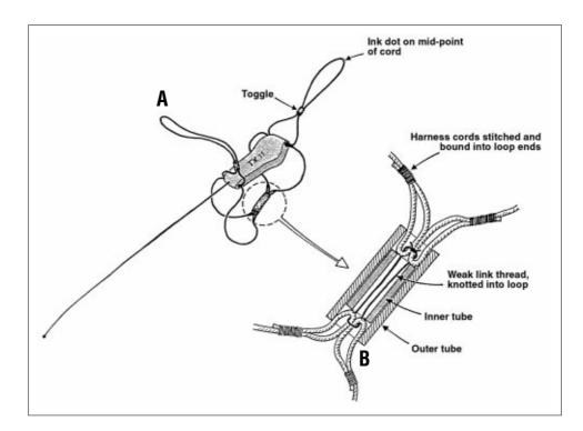
Figure 1. A: Loop formed at either end of transmitter. B: Cord eyelets fit within outer tube.
