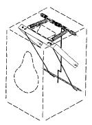
The Timms trap (shown to the left), demonstrated by Paul Jansen, is specifically designed as a kill trap for possums although in some parts of the country the entrance hole, which should be large enough for a possums's head, is too small. As shown here the trap is in the "set-off position; when set the bar is below the entrance hole. While the lure used can be reasonably target specific, the size of the entrance hole makes it difficult to exclude curious non-target species such as weka.
