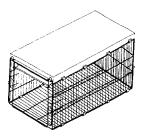
The Edgar trap (to the left), demonstrated by Kim King, was designed specifically to live trap stoats. The cutaway view printed here shows the drop-down door which is tripped by a treadle. The bait is placed between the treadle and the glass end of the box.
