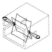
This prototype aluminium box being developed by Bruce Thomas can be used in a variety of ways. Rat, mouse or Fenn (as shown here) traps may be set inside it and pipe extensions to the entrances can reduce non-target species access or improve species selectiveness. This tunnel is far lighter and easier to transport than wooden tunnels but is more labour intensive and expensive to make.
