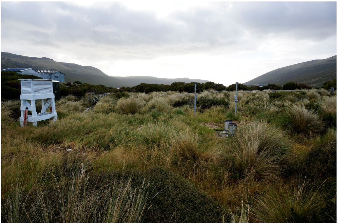
Figure 4. Instrumentation at Campbell Island Automatic Weather Station. Picture taken towards the east. Temperature instruments are located within a Stevenson screen (left), while rainfall gauges and solar instruments can be seen in the centre of the picture. Anemometers attached to a 10 m mast are not shown in this photo. Photo: Andrew Harper.
