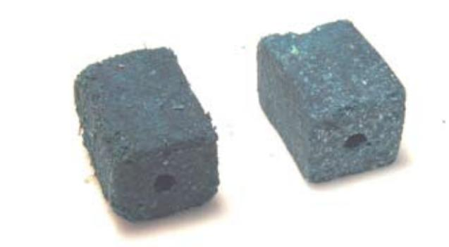
Figure A2.3B. Pestoff® bait weathered for 5 months (on left). The appearance of the bait was similar to bait weathered for 2 and 3.5 months. Unweathered block on right for comparison.
