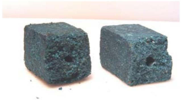
Figure A2.2B. Pestoff® bait weathered for 3.5 months (on left). The appearance of the bait was similar to bait weathered for 2 months. Unweathered block on right for comparison.
