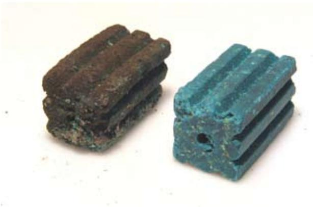
Figure A2.4A. Contrac® weathered for 8 months (on left). Most of the bait's outer surface was covered with brown mould. Other baits were covered with wispy white and powdery green mould. Unweathered block on right for comparison.
