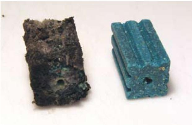
Figure A2.5A. Contrac® weathered for 12 months (on left). Most of the bait's outer surface was covered with brown mould, wispy white and powdery green mould. Unweathered block on right for comparison.
