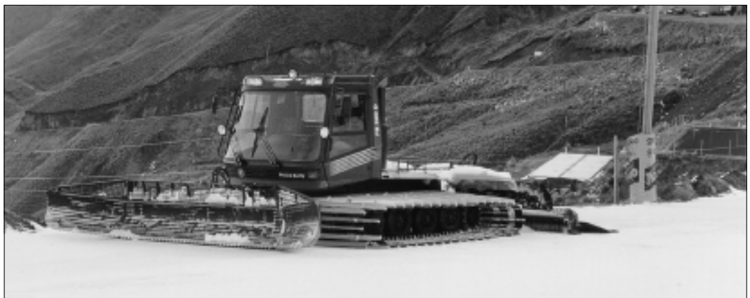
Figure A1.1 One of the three Kassbohrer snow groomers used at Treble Cone Ski Field with attached blade at front and rotary tiller at rear.
