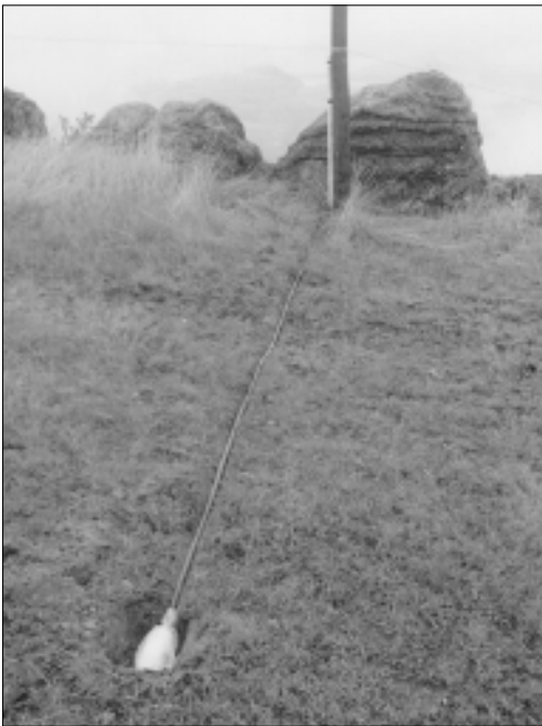
Figure A1.2. Oil-filled rubber hose in position to measure bearing capacity of snow groomers at the learners' slope, Treble Cone Ski Field.
