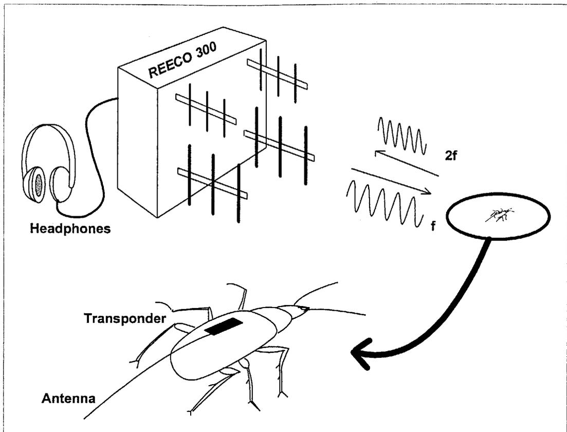
FIGURE 6. REECO™ MODEL 300 HAND-HELD TRANSCIVER UNIT WITH HEADPHONES AND EXAMPLE OF A SMALL TRANSPONDER (HP2835 DIODE AND 3 cm ANTENNA) GLUED TO THE BACK A CARABID BEETLE.
