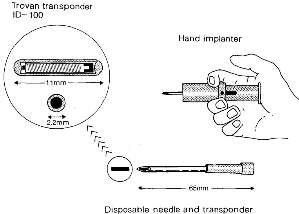
FIGURE 4. TROVAN PASSIVE INTEGRATED TRANSPONDER (PIT), MODEL ID100 AND HAND IMPLANTER WITH STERILE DISPOSABLE NEEDLE APPLICATOR.
