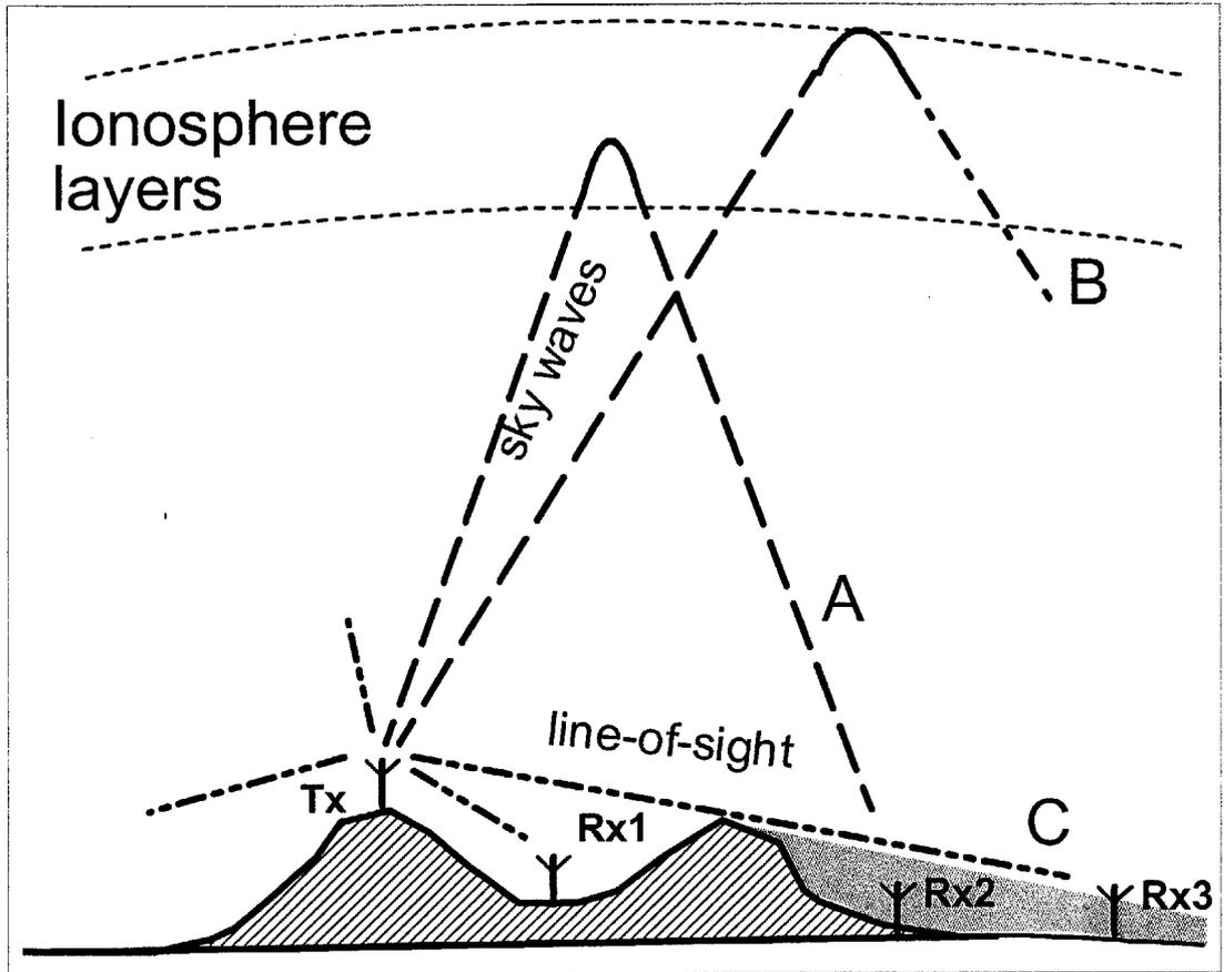
FIGURE 2. RADIO SIGNAL PROPAGATION: EXAMPLE OF HF SKY WAVE PROPAGATION (A & B) FROM Tx TO Rx1-3 AND VHF LINE-OF-SIGHT PROPAGATION (C) FROM Tx TO Rx1 AND Rx3. Rx2 REMAINS IN TOPOGRAPHIC SHADOW TO VHF SIGNALS.
