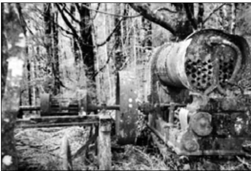
Figure 8. The patent Robey fixed engine.
