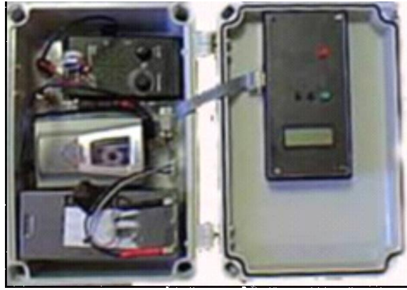
Figure 1. This figure shows one of DOC's automatic bat detection and recording devices (known as an automatic bat monitor or ABM). These units incorporate a voice-activated tape recorder and a timer which enable the unit to be run in the field for several days. The DOC Electronics Workshop should be contacted to find out more about recent developments.
