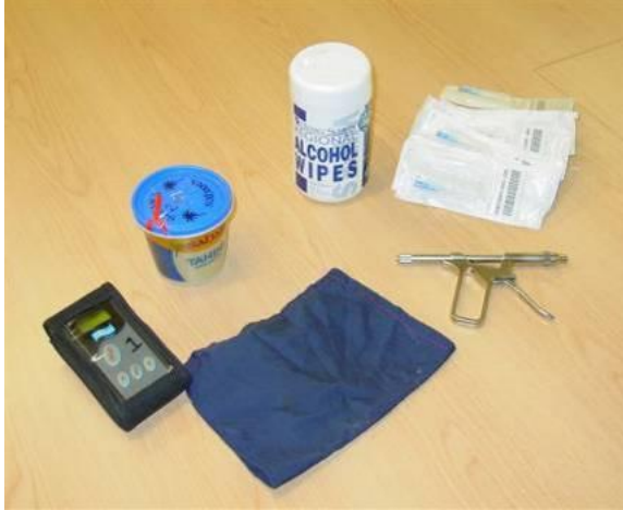
Fig. 69. Some of the main components of a PIT-tagging kit: tag reader, clean bat bag, insertion gun, tags/needles, container to hold used needles and alcohol wipes. Additional essential items are a spare 9-V battery for the reader and recording sheets to record tag and bat details. Photo: J Sedgeley
