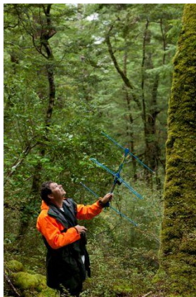
Fig. 78. Tracking a bat with a three-element Yagi aerial. Photo: S Bernert
