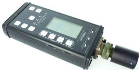
Fig. 7. Examples of hand-held bat detectors that use different methods for transforming ultrasound into audible sound. (A) Batbox Ltd Batbox III D heterodyne detector; (B) Titley Scientific Anabat Scout heterodyne and frequency-division detector; (C) Pettersson Elektronik D1000X heterodyne, frequency-division and time-expansion detector; (D) Wildlife Acoustics Inc. Echo Meter Touch 2 detector with heterodyne and real-time expansion modes (as well as visual output of a full-spectrum spectrogram).
