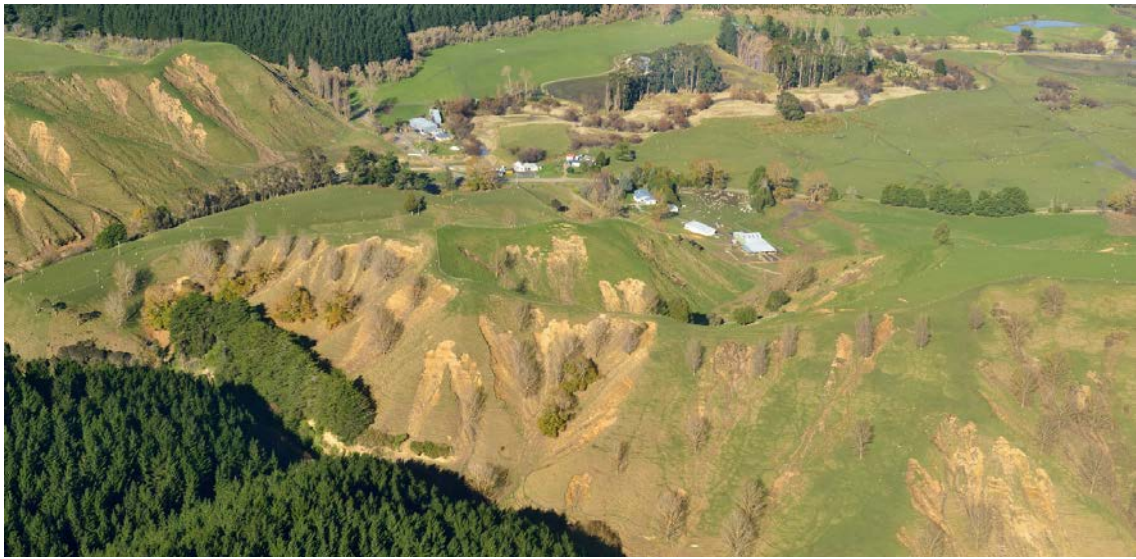
Figure 5-B Slip damage on hill country in the Whanganui catchment. Image © Malcolm Todd
