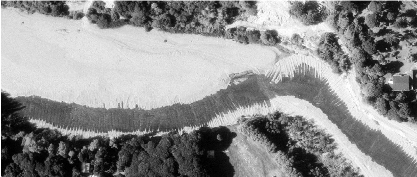
Figure 2-11 Bulldozer tracks where material has been pushed back and forth across the bed to set the river's course, 1986, near XS 370, about 800 m downstream of the old SH1 bridge.
