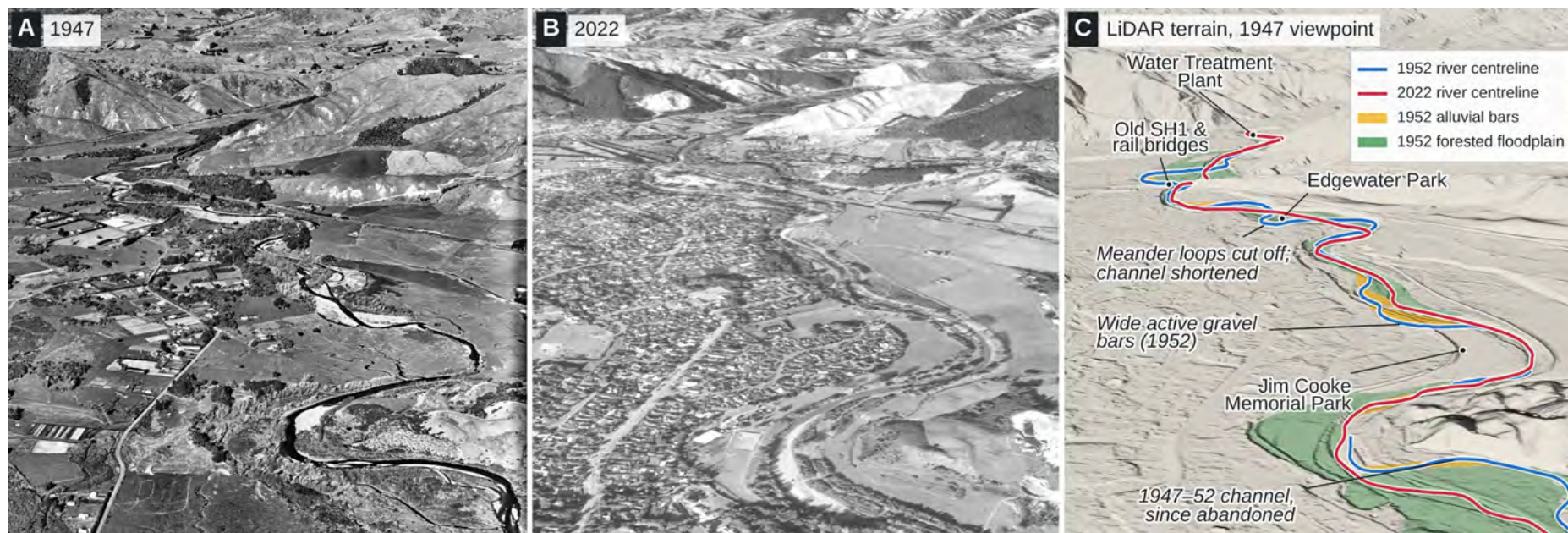
Figure 1-2 The Waikanae River in 1947 (left; Whites Aviation) and 2022 (right). In 75 years the river has changed from a bifurcating channel with a mosaic of bars and floodplain surfaces to a single, straightened and confined channel. This report examines the processes and decisions behind that change.
