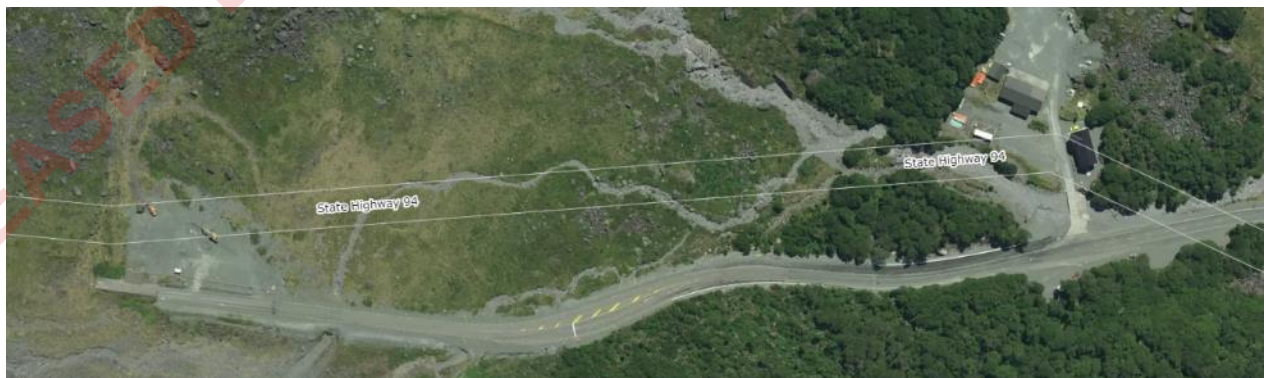
Figure 2: Aerial image showing SH94 Legal alignment versus the physical alignment.
