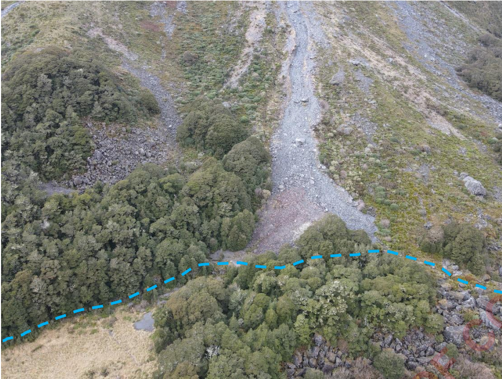
Figure 19: The active debris flow/rock avalanche path on the proposed Gertrude Valley Loop Track.
