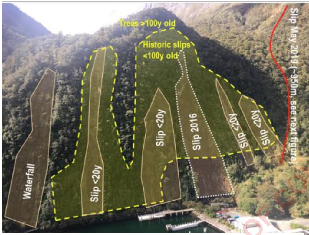
Figure 14: Tree slides and landslides in the hillslope next to freshwater basin in Milford Sound (source: Stantec 2021).
