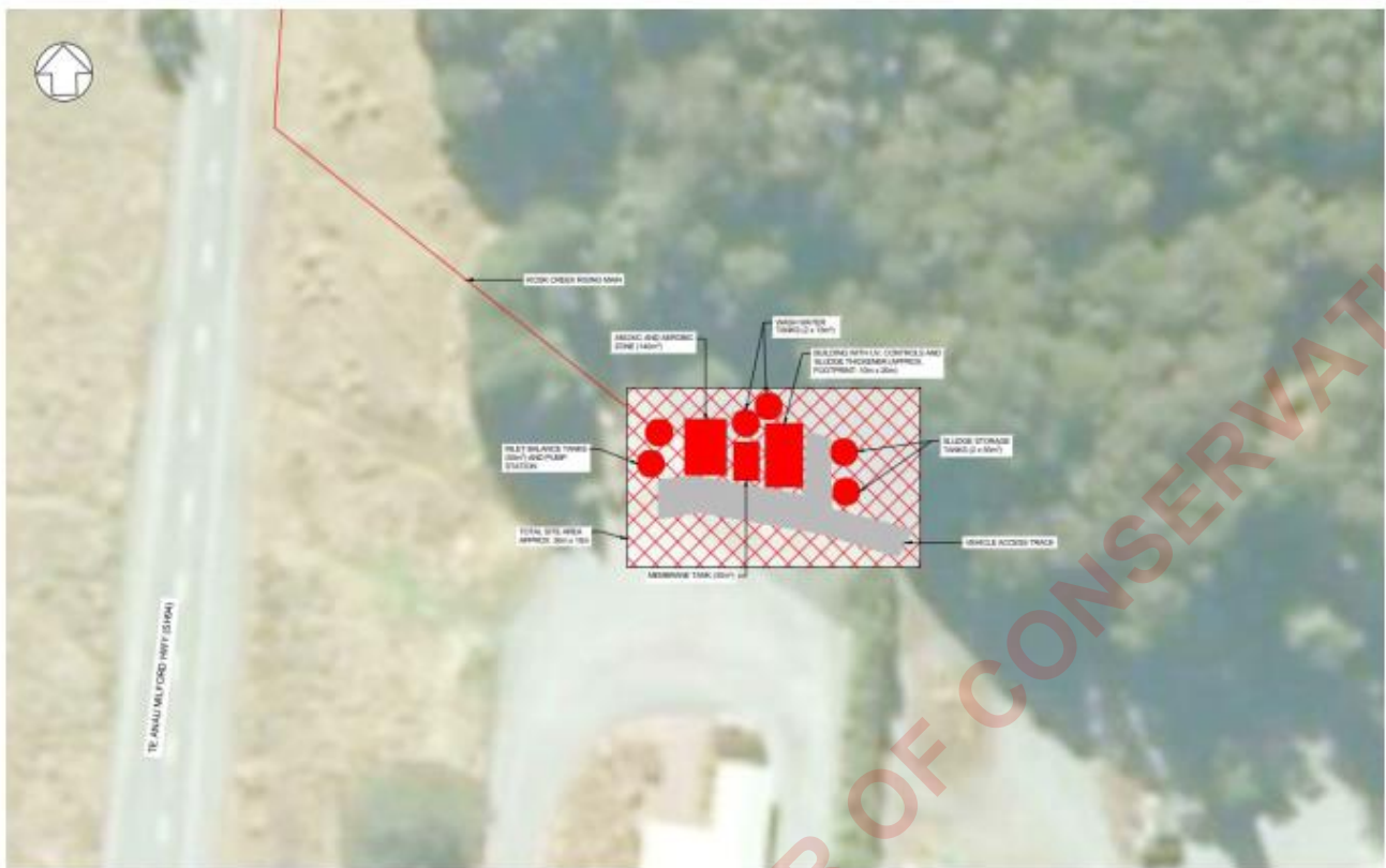
Figure 18: Te Huakaue Knobs Flat indicative wastewater treatment plant layout
