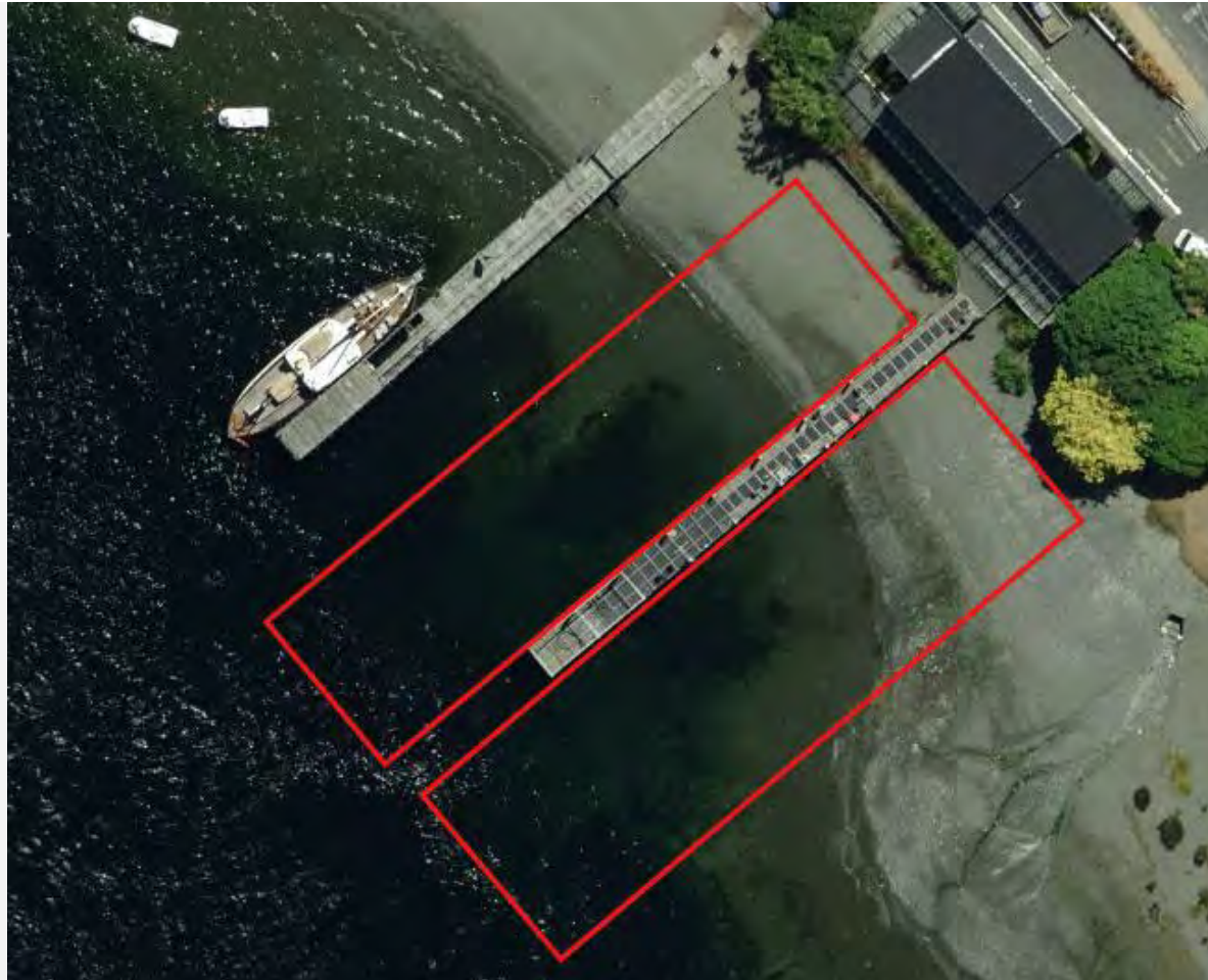
Figure 37 – aerial photo showing approximate larger area that needs to be utilised to berth vessels at Te Anau Lakefront jetty
