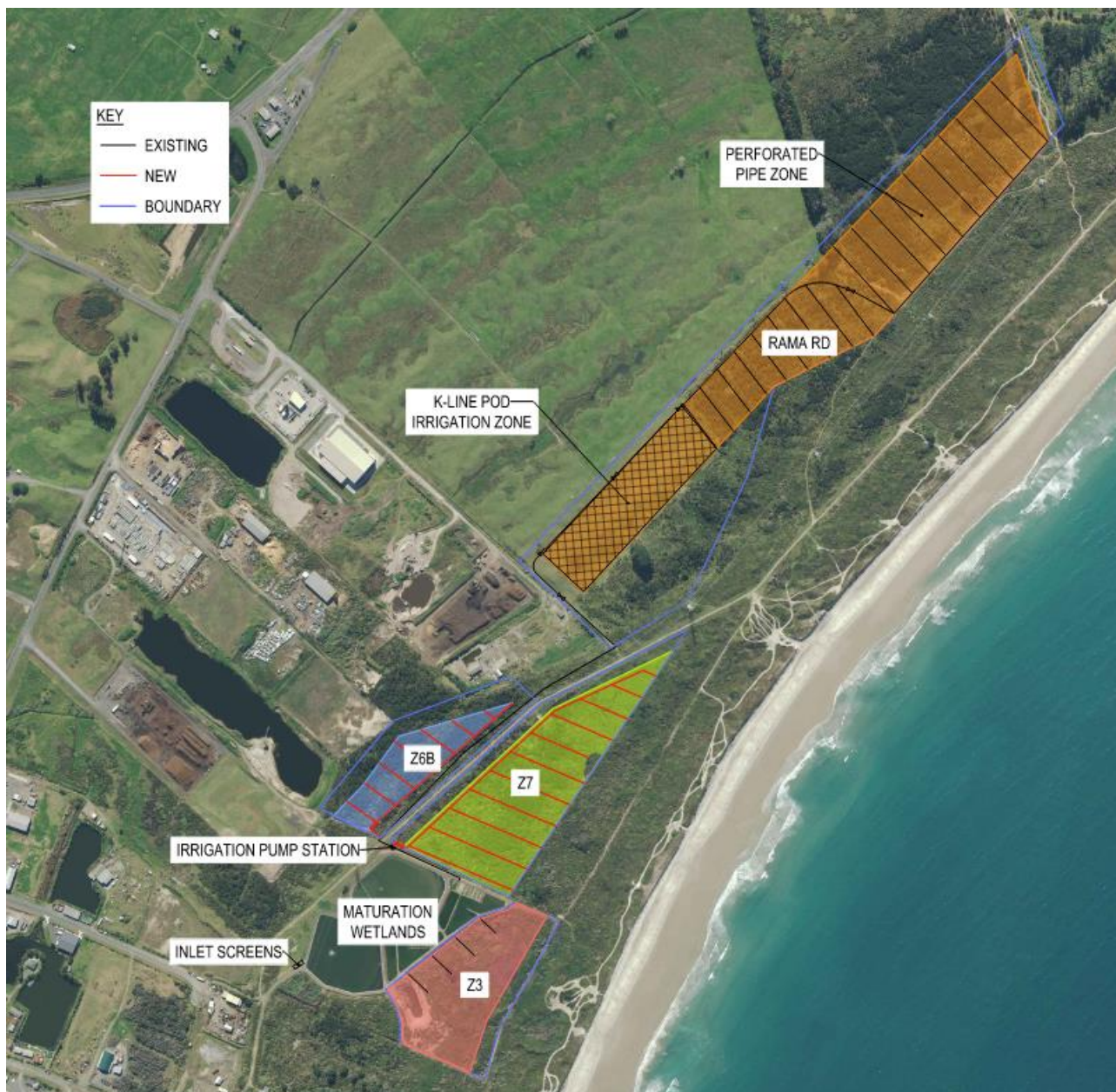
Figure 11: Image showing example of proposed irrigation layout for Workstream Three: Zone 6B + Zone 7 + Zone 3 (refer to Concept Design Report for other scenarios). Lateral application lines are shown in black (existing) or red (new).
