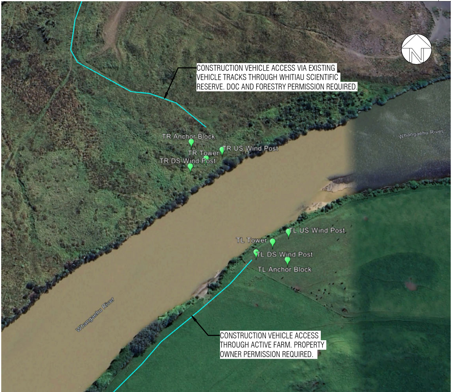
Figure 2: Approximate layout of bridge foundations. Final locations to be set-out by Contractor and approved by Engineer before construction.
