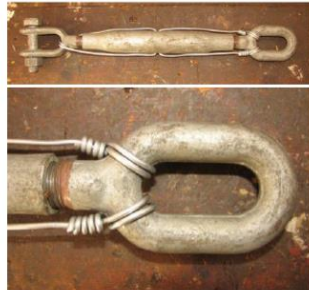
6 - Terminate wire at end-fitting as shown steps 1 - 3
