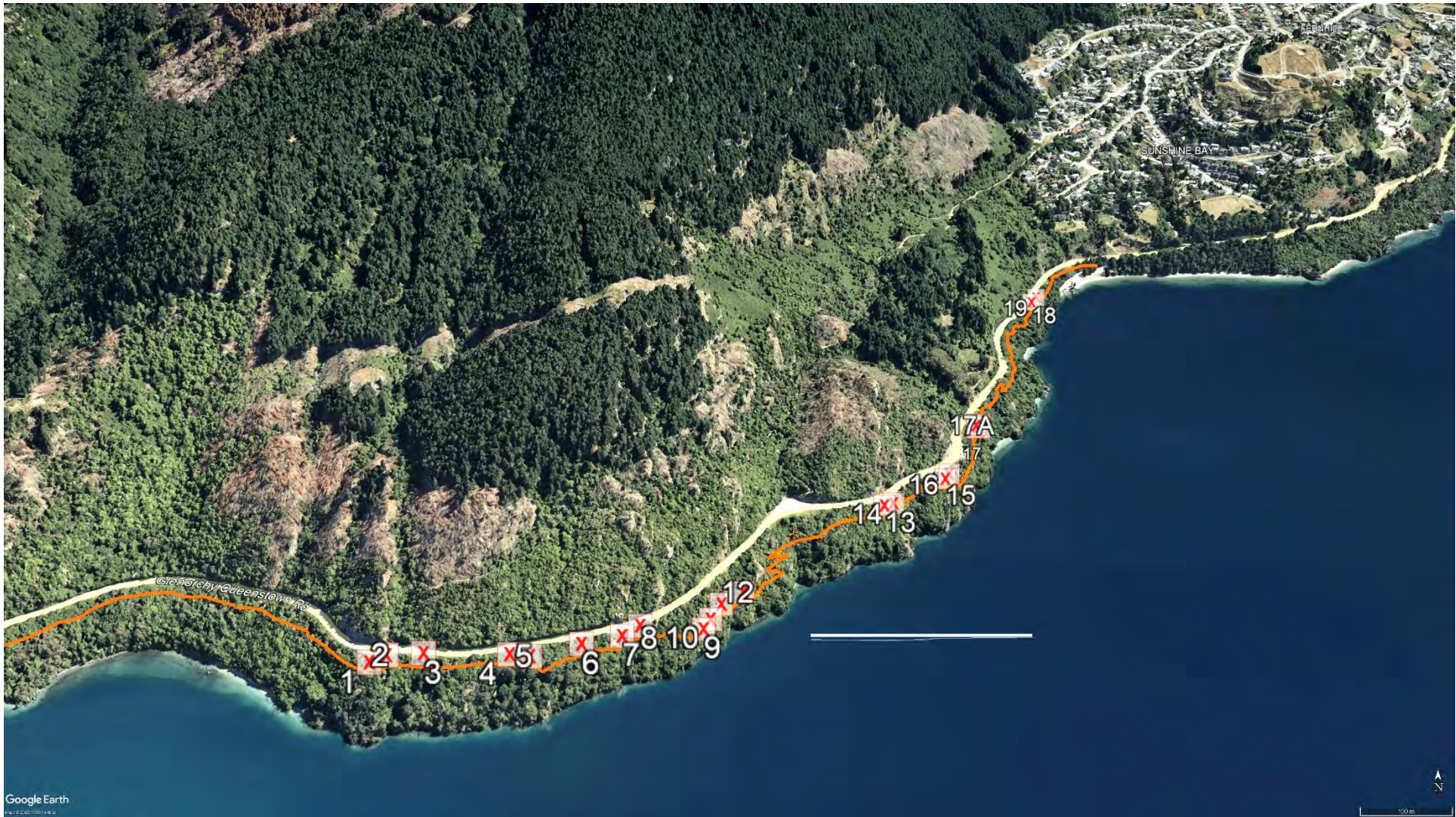
Plate 40: Areas identified by Elevate Trail Building as requiring rock breaking/ blasting to install the trail between Sunshine Bay and Five Mile Creek. Refer Table 7 for the estimated dimensions of each rock breaking/ blasting site. A total length of at least 280m of rock breaking/ blasting identified; a 280m line shown to indicate length. The popular rock jumping site known as “Little Thailand” is near WP17
