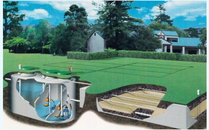
Modern septic tank, sand filter and drip irrigation field
