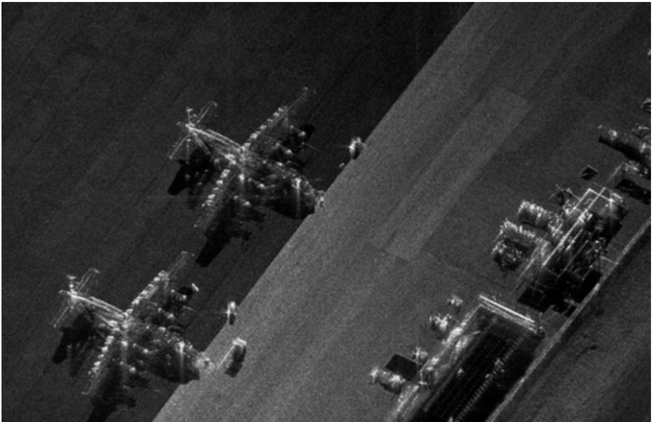
Figure 1 – Airport imaged using UWB SAR
