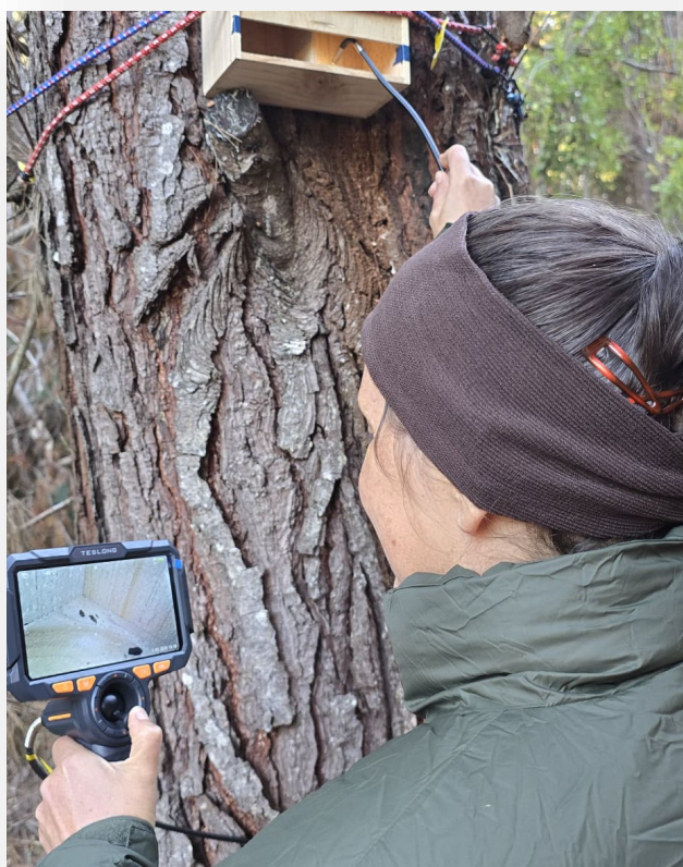
Figure 1. Inspecting a temporary artificial bat roost box for signs of bats using a Teslong Endoscope with 6mm head. Note bat droppings can be seen in the corner of the box on the Endoscope's screen. (photo credit – Ian Davidson-Watts)
