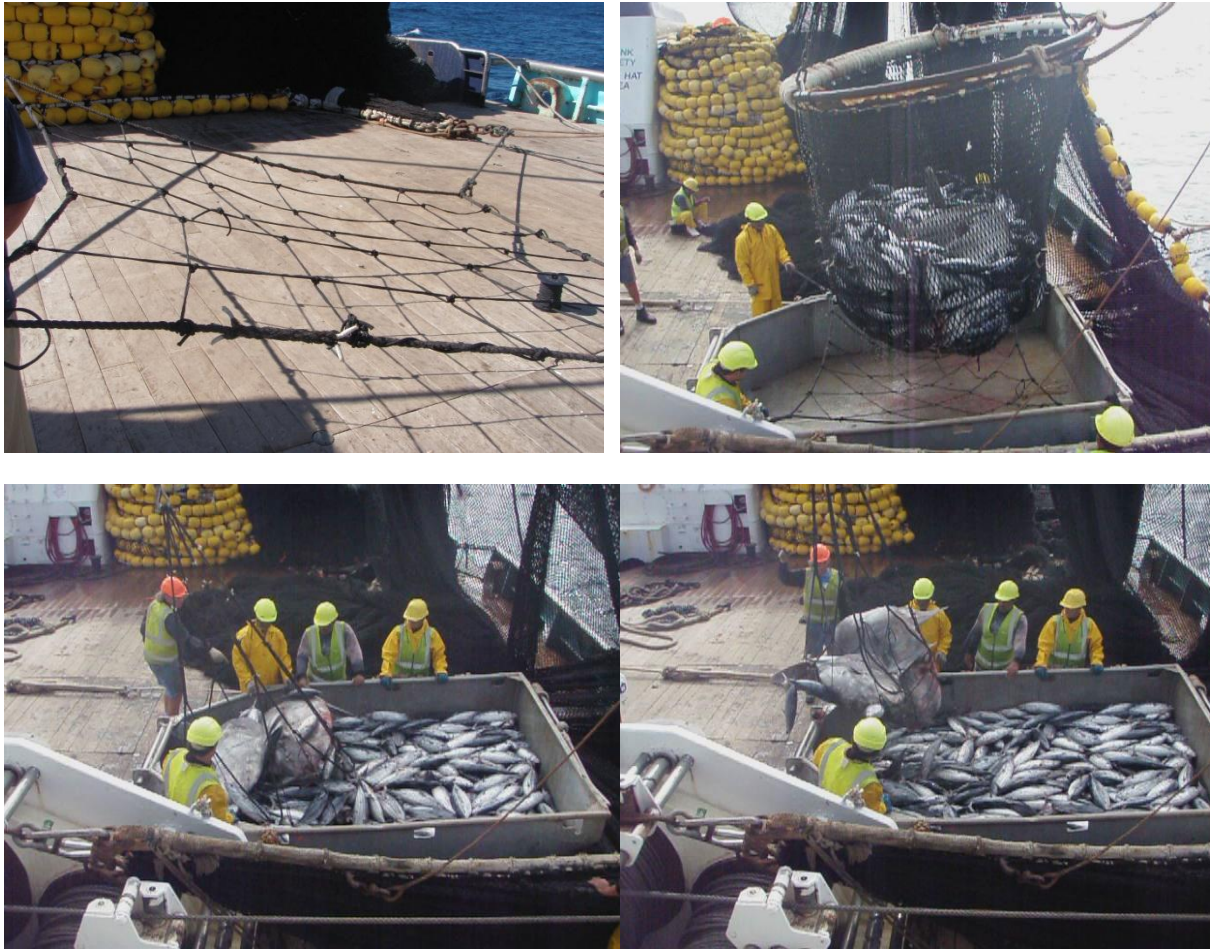
Figure 5. The cargo net used onboard the superseiner, San Nanumea for return of large bycatch over the side (top left). Photographs show a brail net containing target species and two sunfish being brought onboard (top right); the brail is released and the cargo net used to catch the sunfish (bottom left and right)
