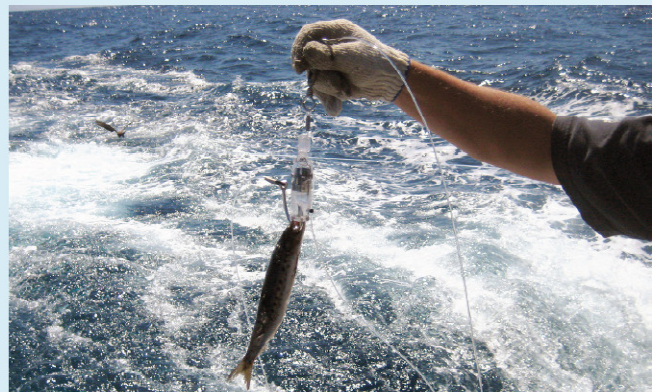
The hook pod loaded with a baited hook on setting. Photo: B. Sullivan
