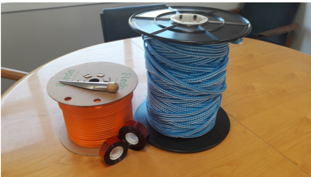
Figure 1: Kraton Aurora Pink 6mm diameter tori line dropper material (aka “the pink stuff” as supplied to vessels.
