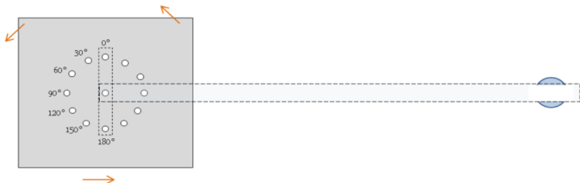
Figure 4. Top view of the measurement apparatus, showing the apparatus reference rotation angles and hydrophone mounted in blue tube (right).
