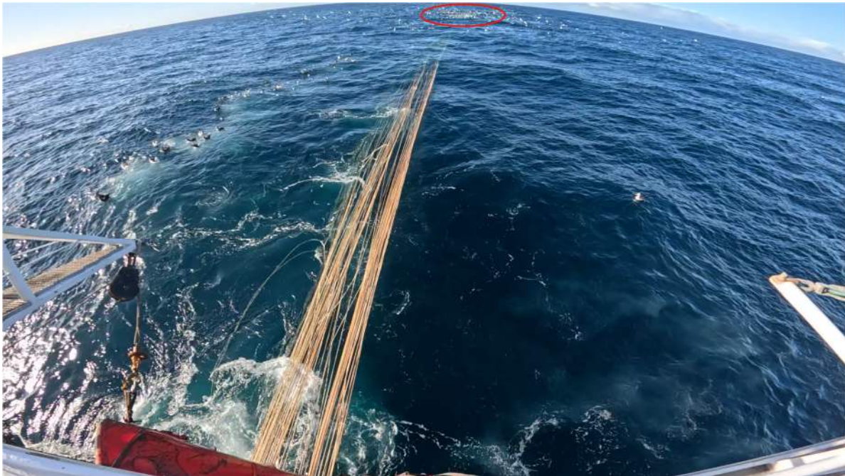
Figure 6. Midwater net being hauled, showing how far from the stern the codend surfaces.
