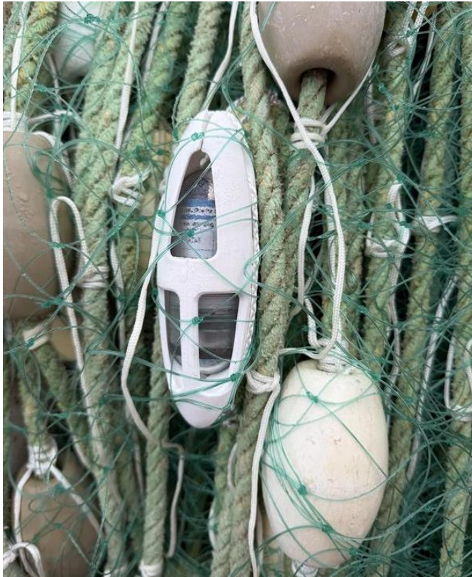
Figure 3. Netguard Fingers attached to the float-line of a 250 m set net, prior to deployment, showing that the devices were lashed securely to the float-line, without any shrouding or insulation, as per manufacturer instructions.
