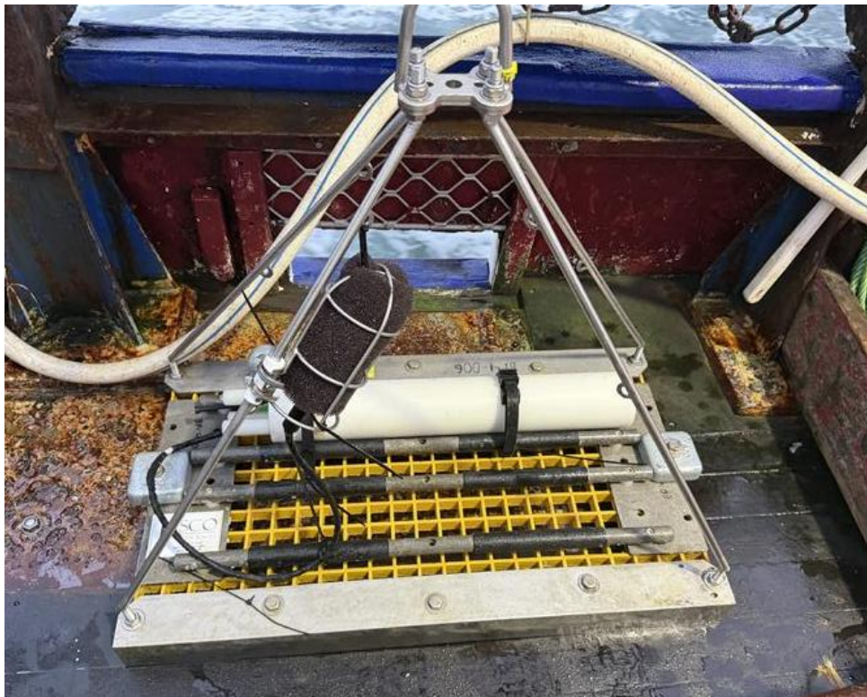
Figure 1. The baseplate JASCO AMAR utilised as the static recorder.
