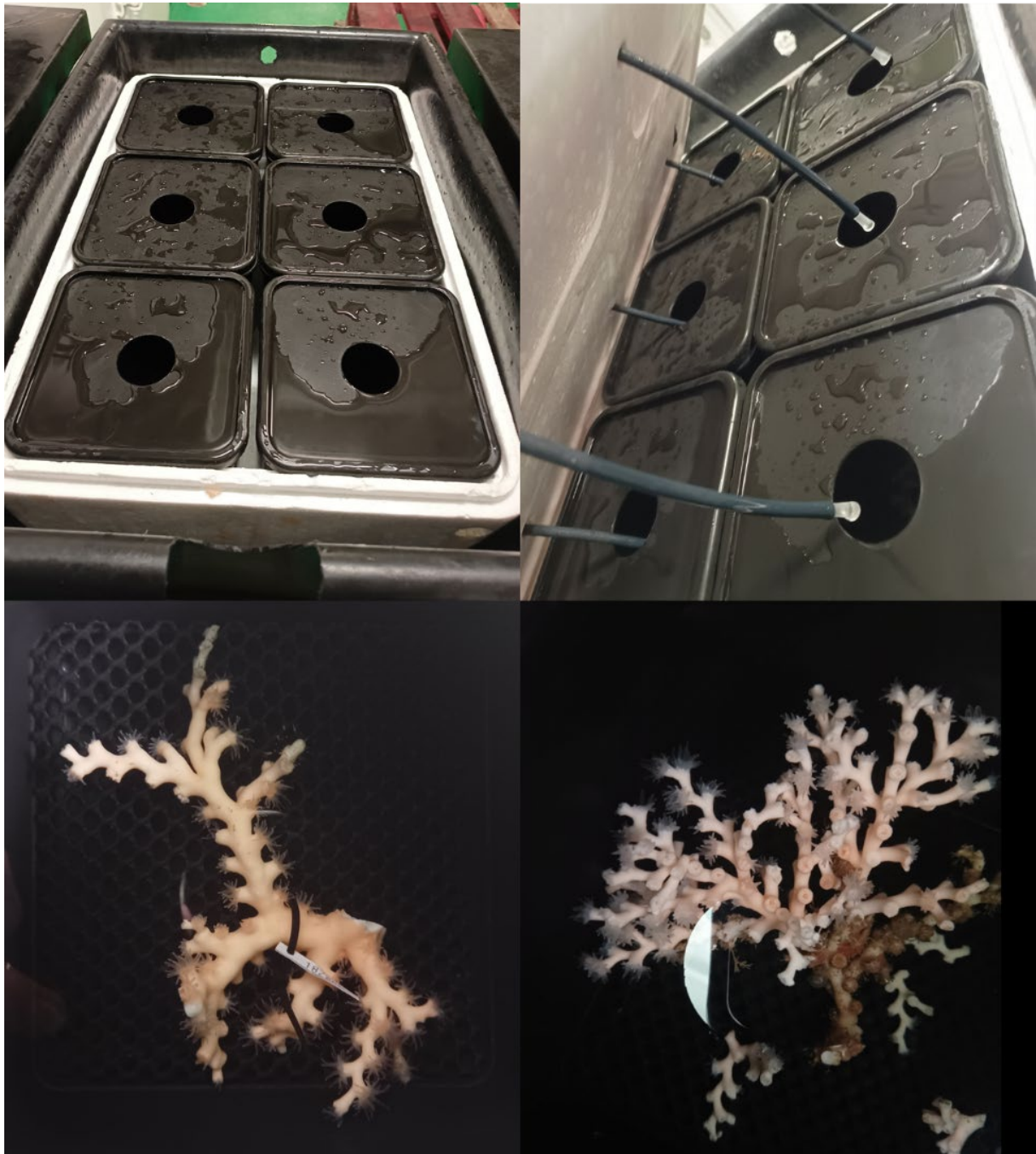
Figure 4-4: Aquarium set-up onboard RV Sonne . Inside each insulated polybin were 6 x 4 L black plastic tanks (top left), each with a dedicated water supply of chilled water via a silicone tube (top right). Bottom images show coral colonies ( Madrepora cf. oculata ) inside 4 L tanks, both with their polyps extended.
