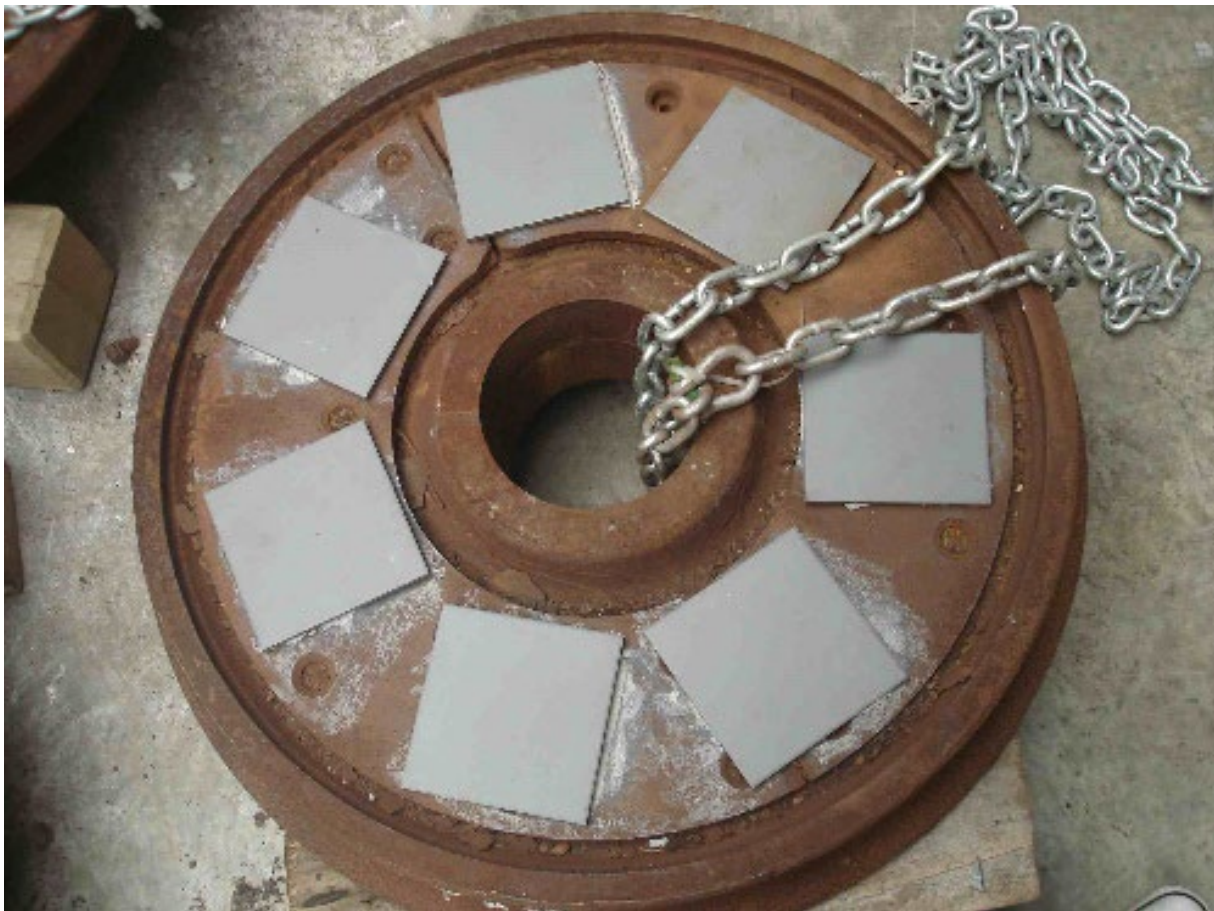
Figure 3-11: Wagon wheel prior to deployment. Grey squares are settlement panels that were attached to the wheels to study settlement and recruitment of deep-sea fauna (see Clark et al. 2021).
