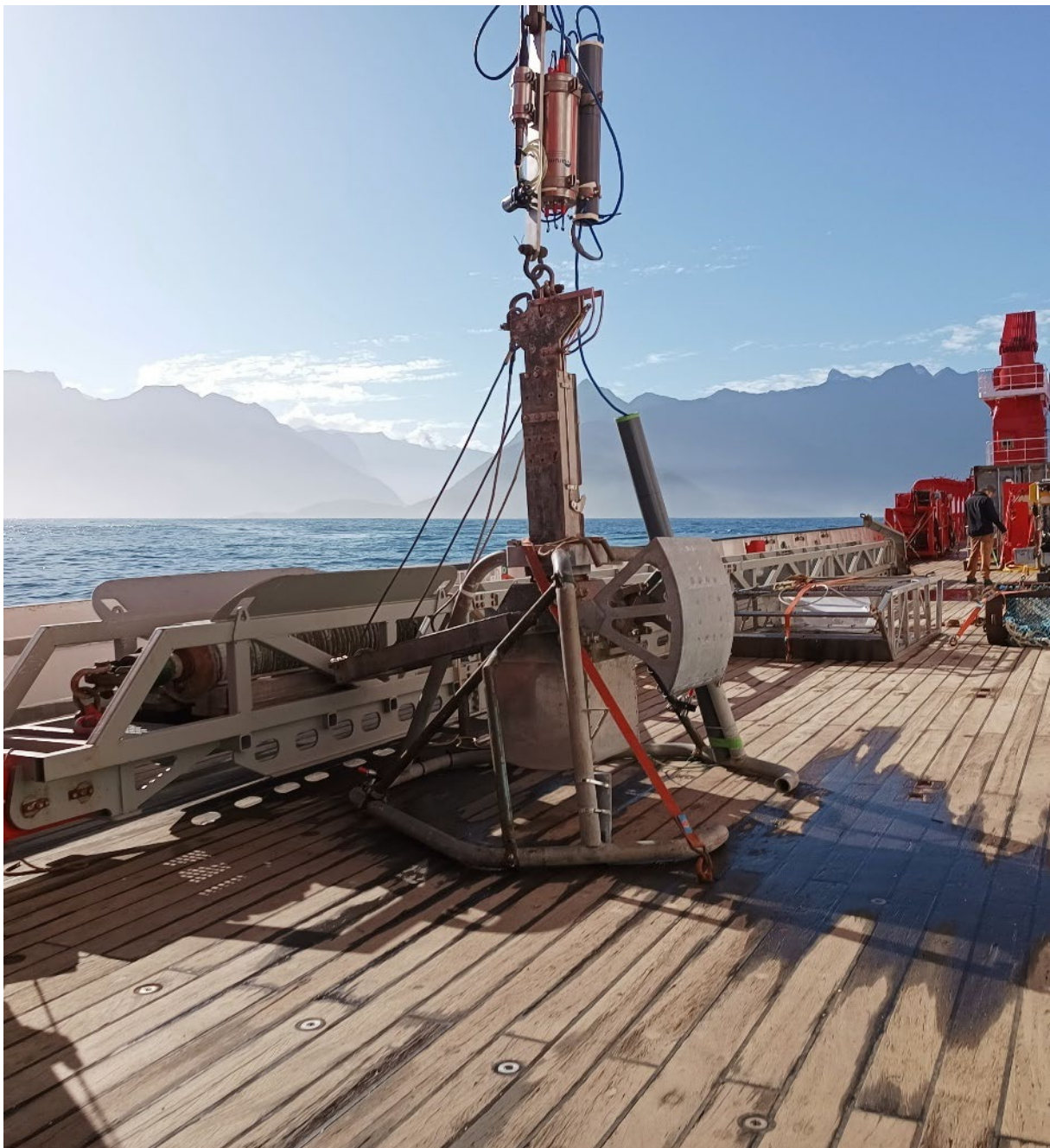
Figure 1-8: TV-guided box corer on deck of RV Sonne . Equipped with a video camera mounted next to the sampling box.
