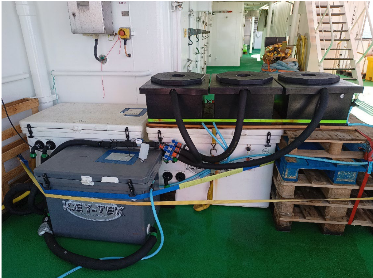
Figure 4-3: Aquarium set-up onboard RV Sonne. The aquarium consisted of a chiller unit (white unit back left), a sump (grey unit at the front) and three aquaria, each with 6 small animal tanks inside. Two water supplies are connected to the system: a high flow of water to the chiller system and a low-pressure feed of clean, filtered, water to the sump. The sump water is cooled by the chiller unit before being circulated to the three aquaria containing animals.
