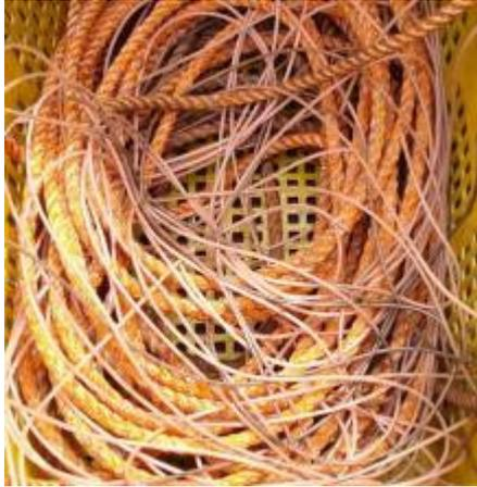
Figure 2. The luminous tubing typically used in streamer lines currently deployed on trawlers  $\geq 28$  m operating in New Zealand waters. Figure 1(a) shows this material when new. Here, the material is shown after 10 days at sea, highlighting the extent of fading that occurs in relatively short timeframes.
