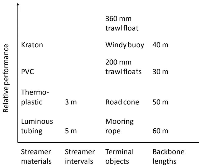
Figure 6. Relative performance of streamer line components tested at sea. Performance was assessed based on characteristics described in Table 2.
