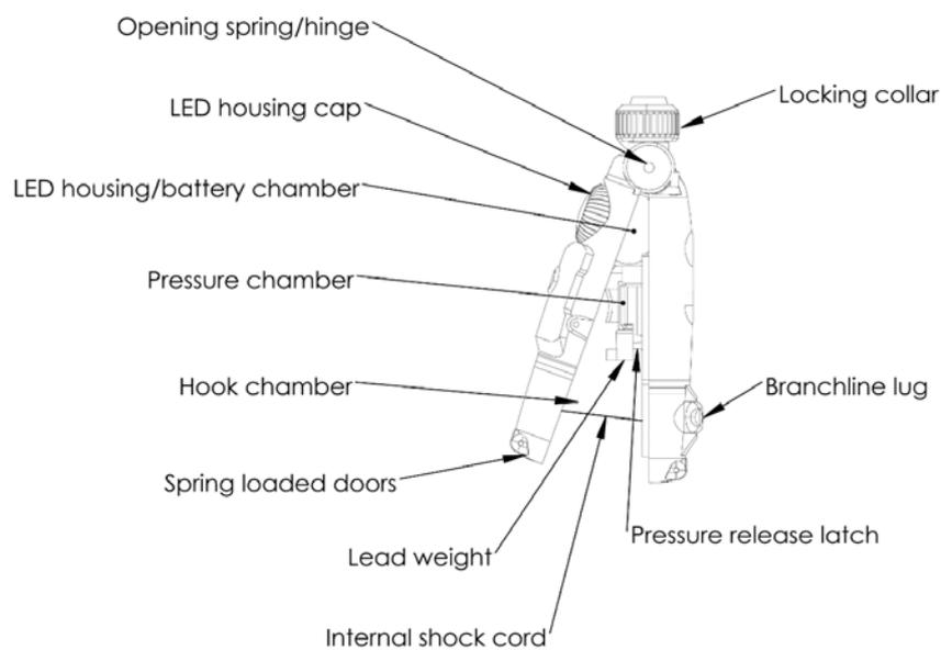
Figure 1. Components of the Hook Pod (NB the diagram depicts a version of the pod with the LED included, the version used in the New Zealand trials (see below) did not contain the LED components)
