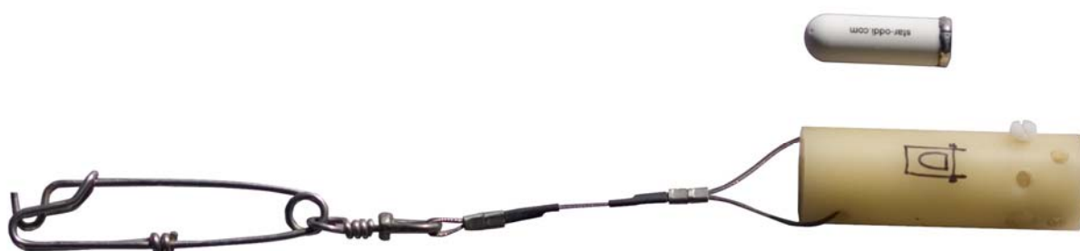
Figure 6 TDR and housing, total length including clip is 32cm.
