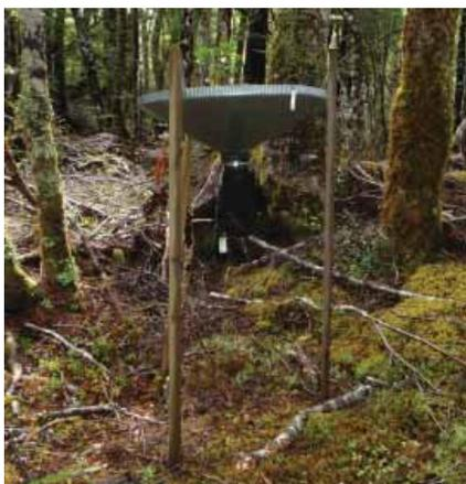
Is that a landed UFO? No, just one of the 40 seed trays used to measure the amount of seed produced by the beech trees.
