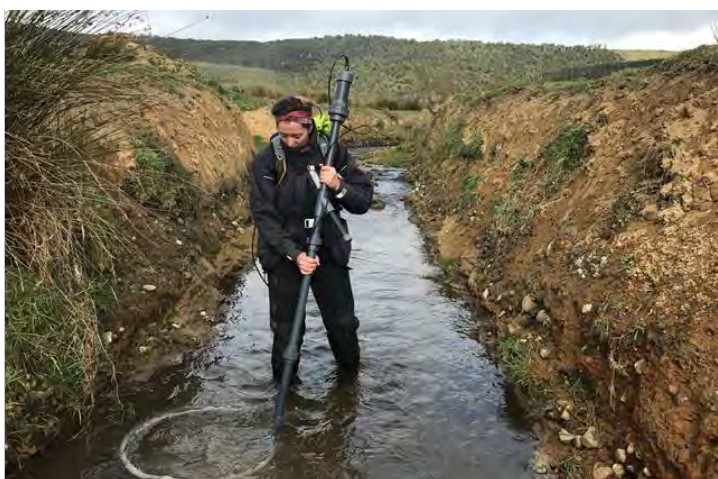
Figure 5-8: Basic search method using the portable PIT system in a stream channel.
