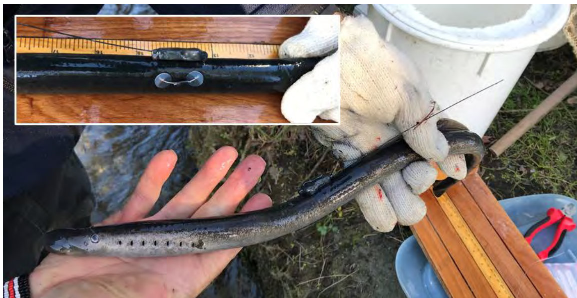
Figure 5-7: ATS external radio tag (F1960) mounted on an adult lamprey. Inset shows the attachment harness.
