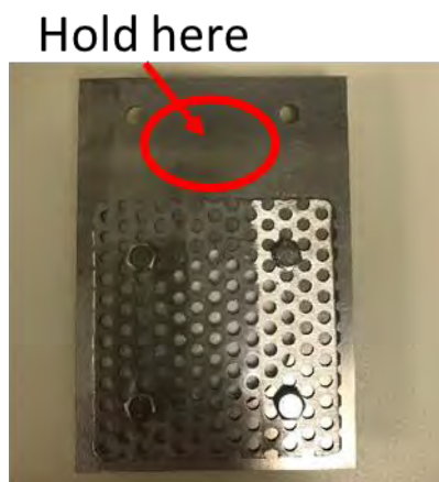
Figure B-1: POCIS samplers used for stream sampling of lamprey pheromones.
