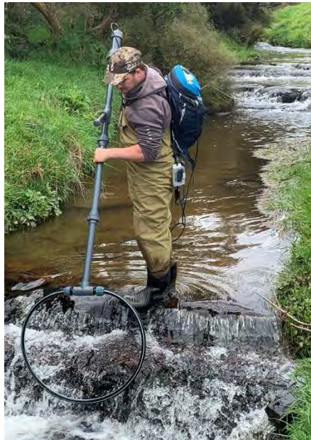
Figure 5-9: Portable PIT system search method for waterfalls and weirs.
