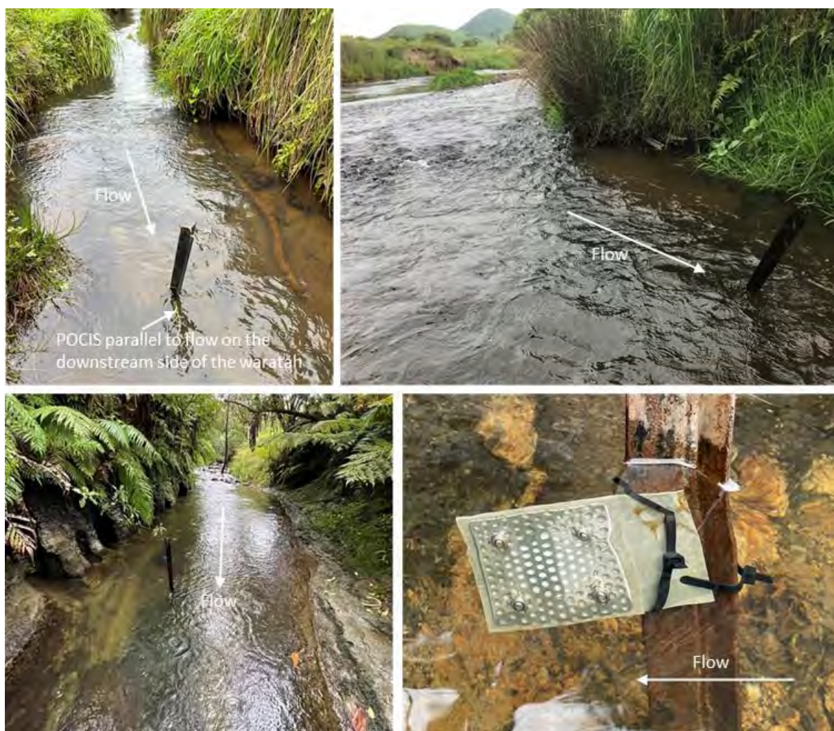
Figure B-2: Picture of POCIS sampling position within small streams (left top and bottom) and a large river (top right). Cable tie configuration depicted bottom right. White arrow indicates direction of flow.
