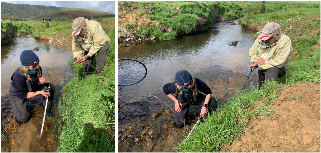
Figure 5-16: Verifying a dropped PIT tag in finer substrates using the stick antenna.
