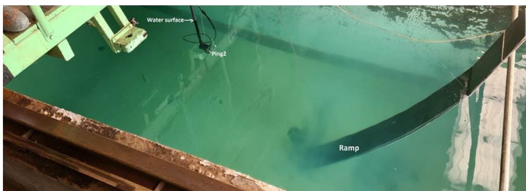
Figure 3: Top – Camera Positioning System (CPS) hardware and (middle) application software embedded in the existing detection module. Bottom – The test system simulating a rising bed with a flexible ramp.
