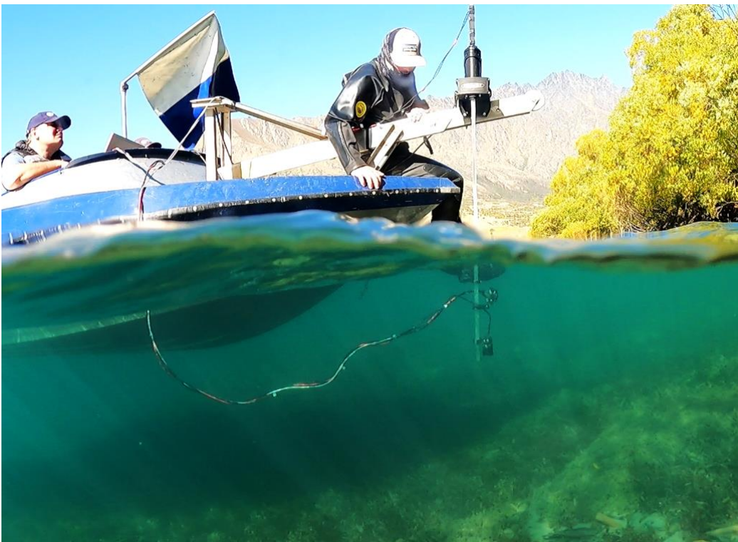
Figure 5: Initial trial of the CPS in the Kawarau River, March 2024. Underwater and topside view of the GoPro camera approaching the river edge.
