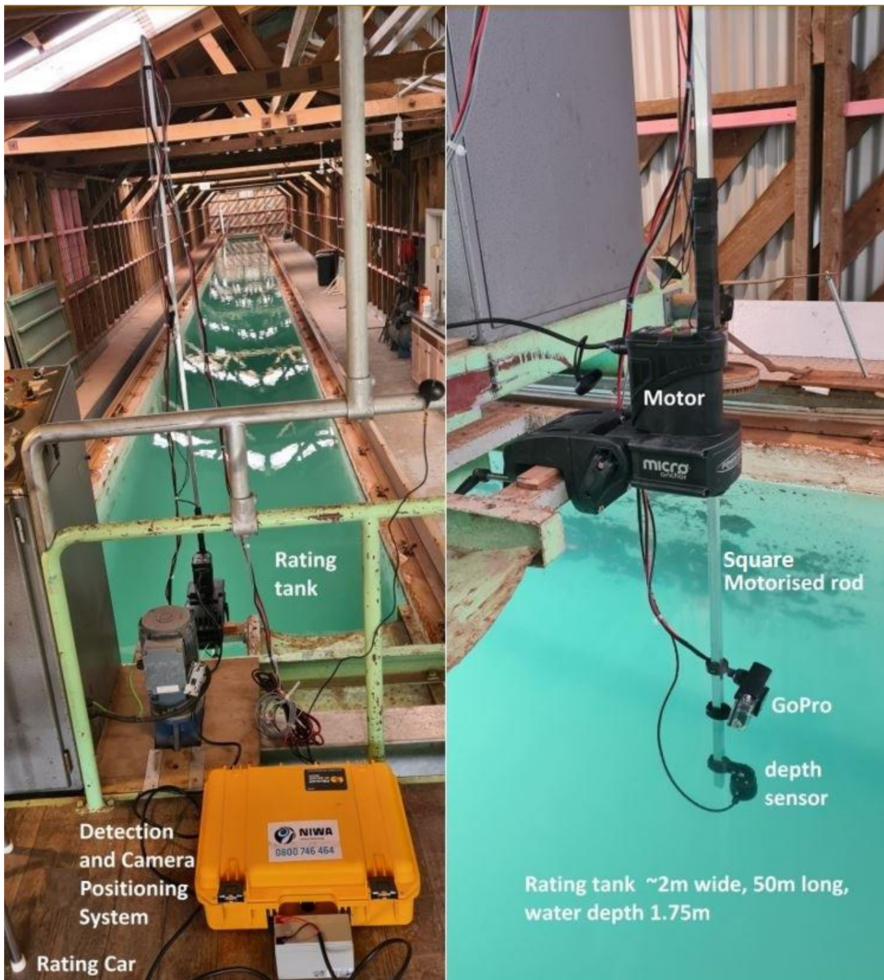
Figure 1: Left – The Camera Positioning System (CPS) equipment mounted on the rating car in the flume. Right – The modified motorised rod that raises and lowers the GoPro video camera.
