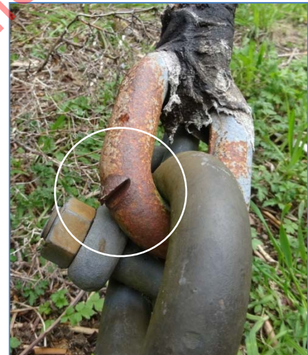
Figure 5.36 Cut in rigging screw eye (possible crack propagator)
