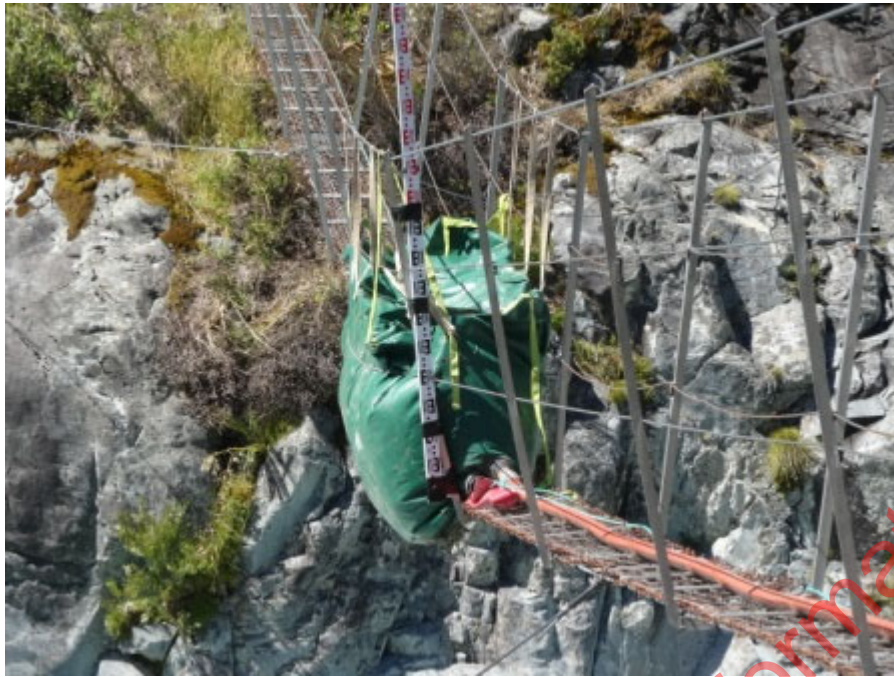
Fig 5. Test bag straps not tight enough on hand cables causing bag to flop over side of deck
