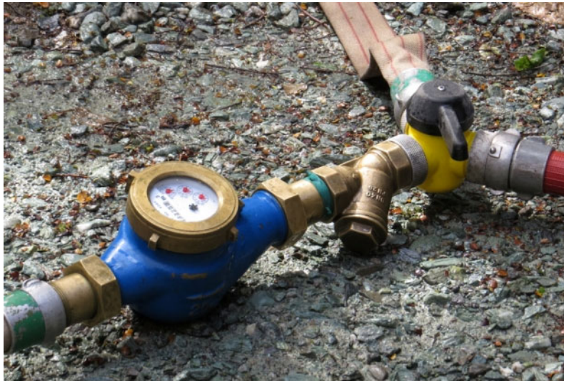
Fig 6: Flowmeter with splitter/divertor
