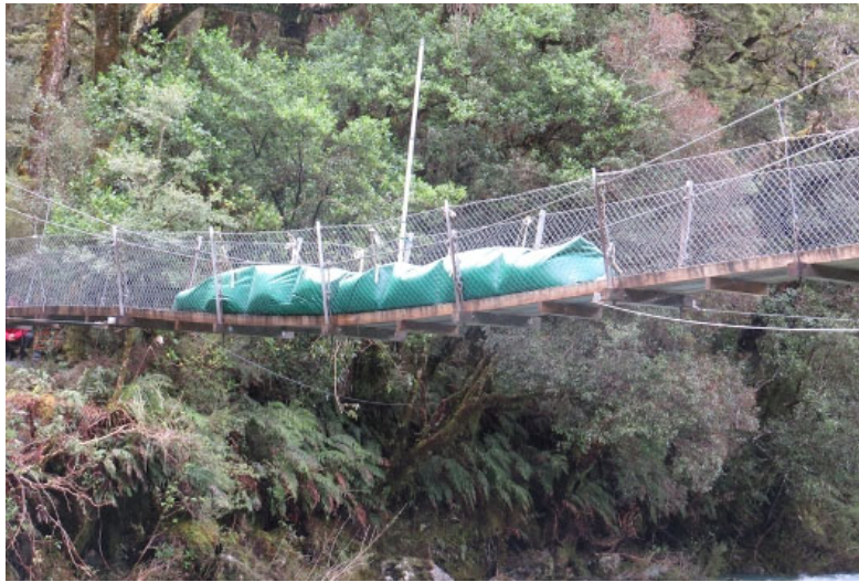
Fig 14: Larger 2500kg test bag for load limit of 2 or more persons
