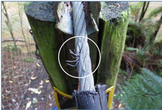
Figure 5.41 Wires cut (windfall impact) near cable saddle
